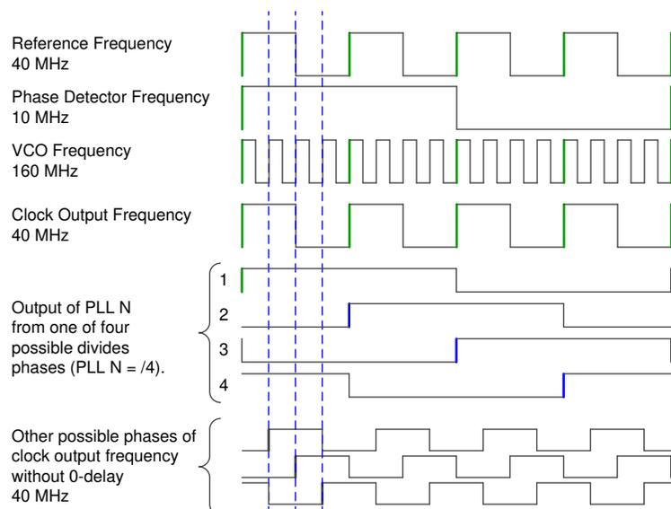
**Figure 8. Timing Plot for ZDM with Phase determinism**
