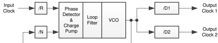
Figure 6. PLL Block Diagram with Clock Distribution
