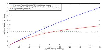
Figure 4. Estimated Battery Life Comparison: Nanotimer vs. MCU Standby Mode
