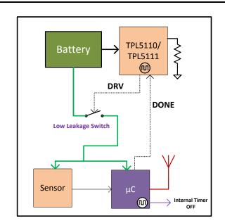
Figure 2. A Sensor Node with an Integrated Powergating System Nanotimer
