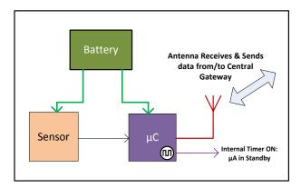
Figure 1. A Typical Sensor Node
