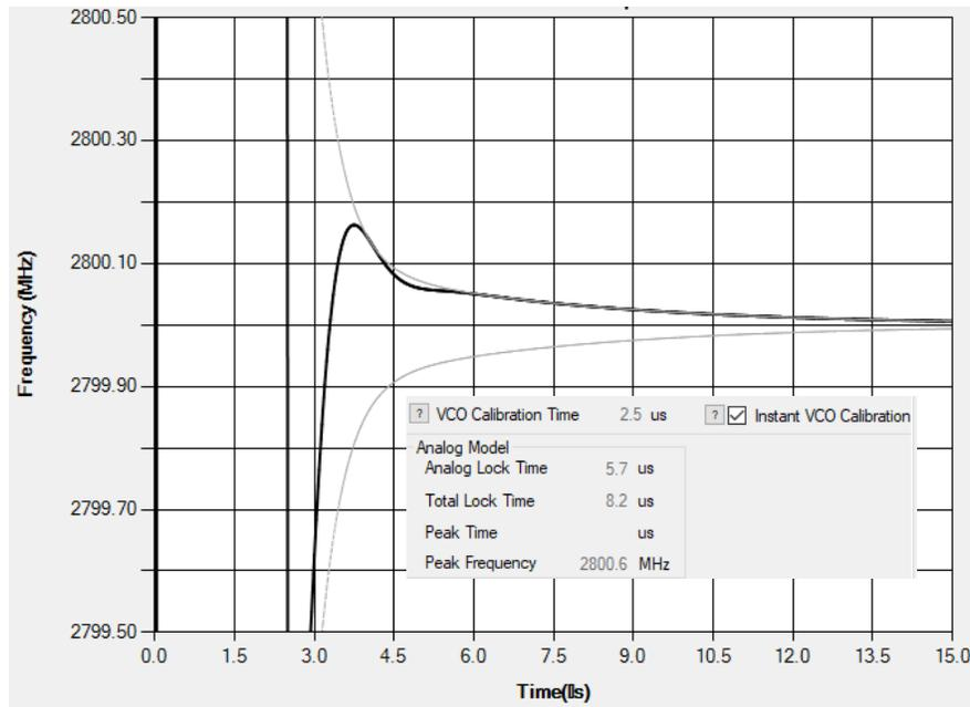
Figure 4-4. Lock Time Simulation
