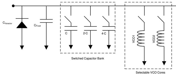
Figure 2-1. Simplified Tank Circuit for Silicon VCO
