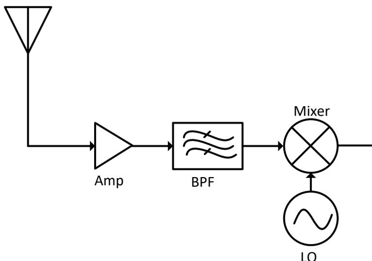
**Figure 1-1. Typical Receiver Architecture**
