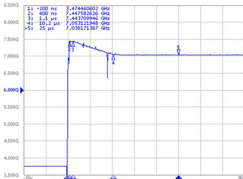
**Figure 3-2. LMX2594 VCO Calibration With Partial Assist**
