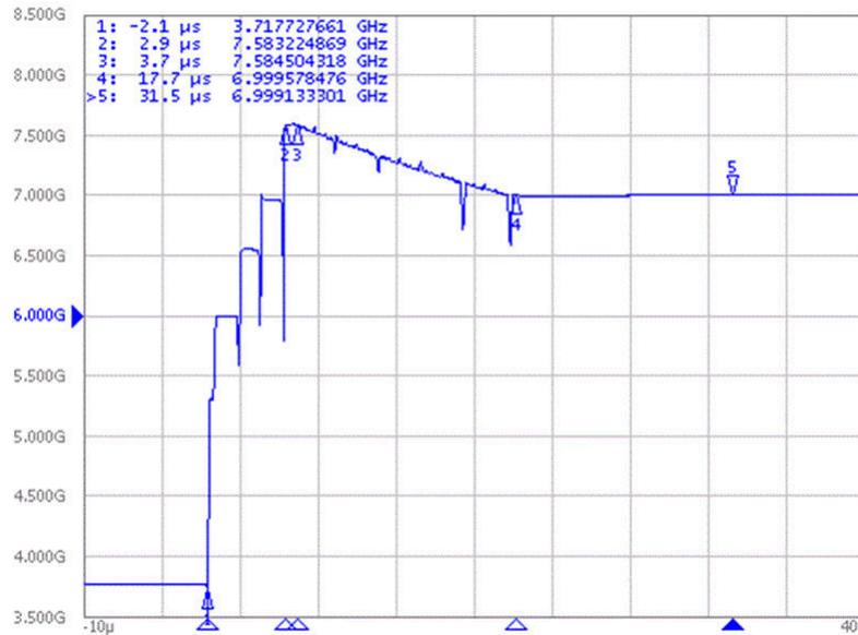
**Figure 3-1. LMX2594 VCO Calibration With no Assist**
