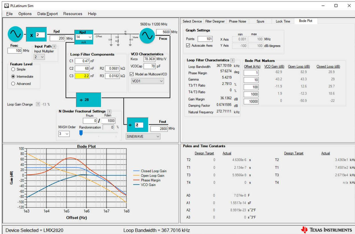
Figure 4-3. Loop Filter Setup
