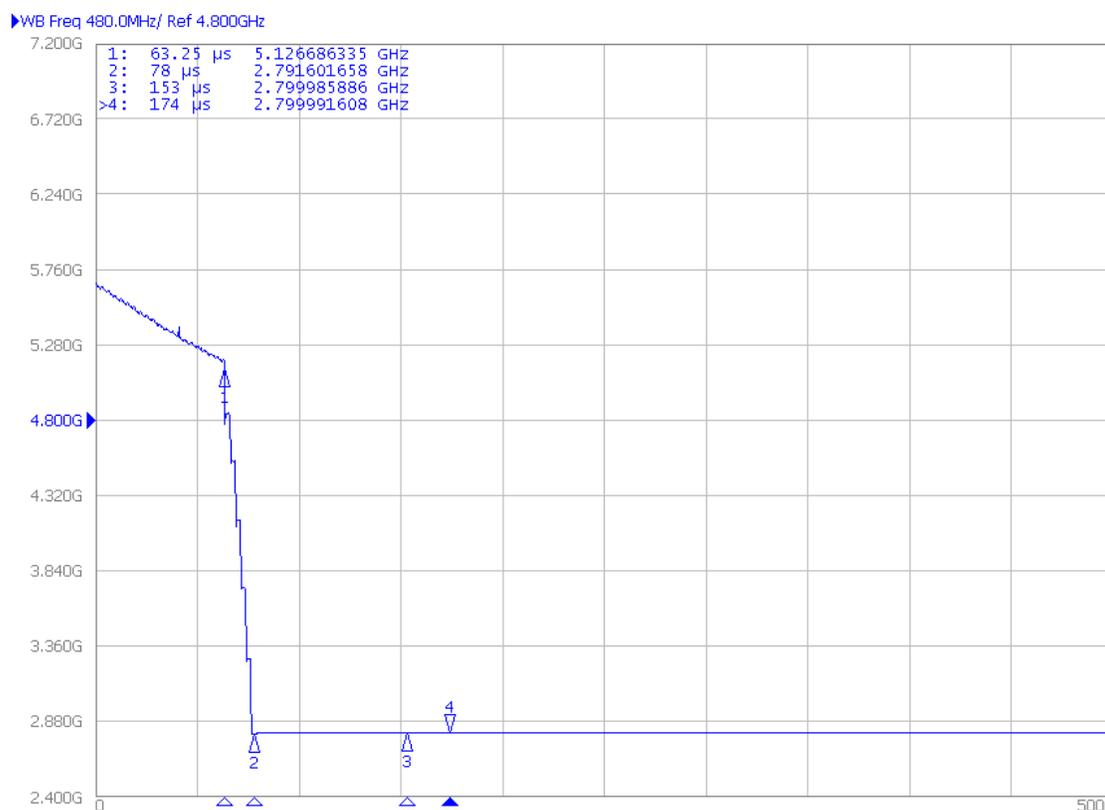
Figure 4-1. LMX2820 Unassisted Lock Time
