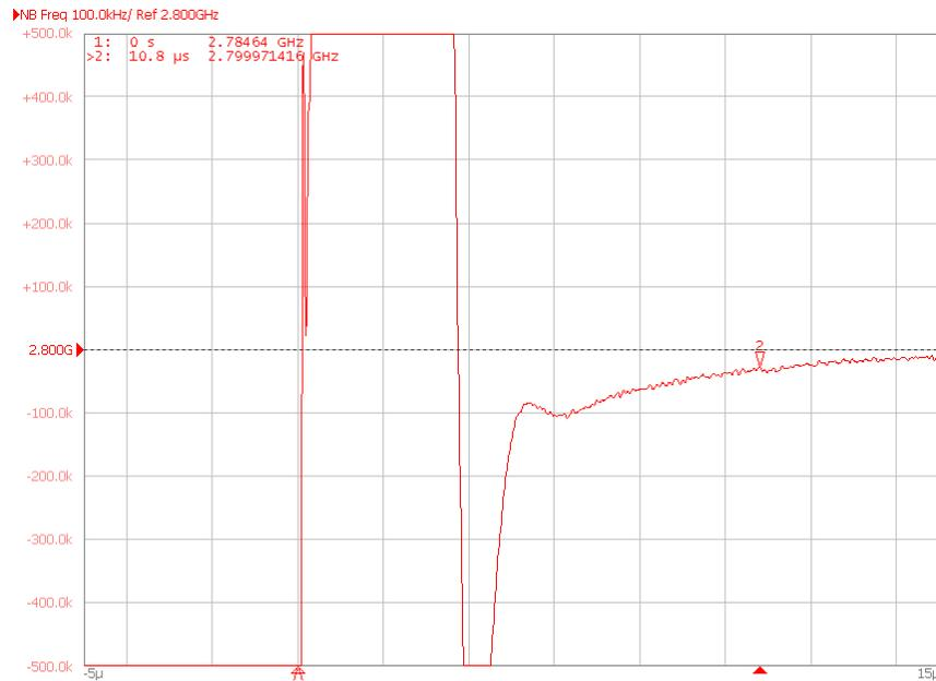
**Figure 4-6. Narrow Span Instant Calibration With the LMX2820**
