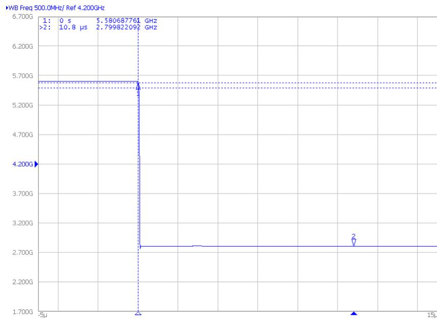
Figure 4-5. Wide Span Instant Calibration With the LMX2820
