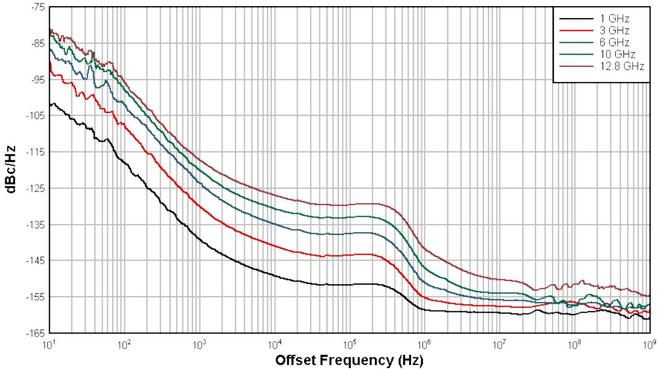
**Figure 2-2. Cascaded LMX1204 Phase Noise Measurements**
