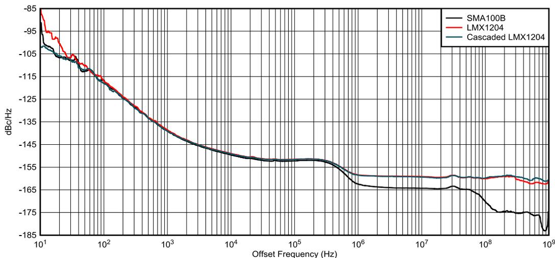
**Figure 2-3. Phase Noise Comparison - 1 GHz**
