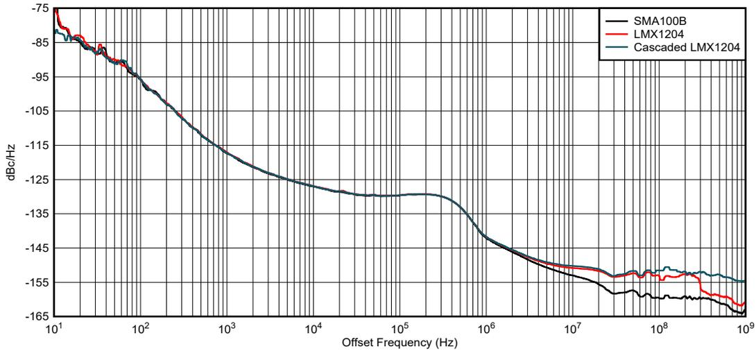
**Figure 2-7. Phase Noise Comparison - 12.8 GHz**
