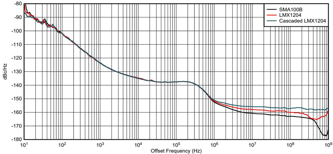
**Figure 2-5. Phase Noise Comparison - 6 GHz**
