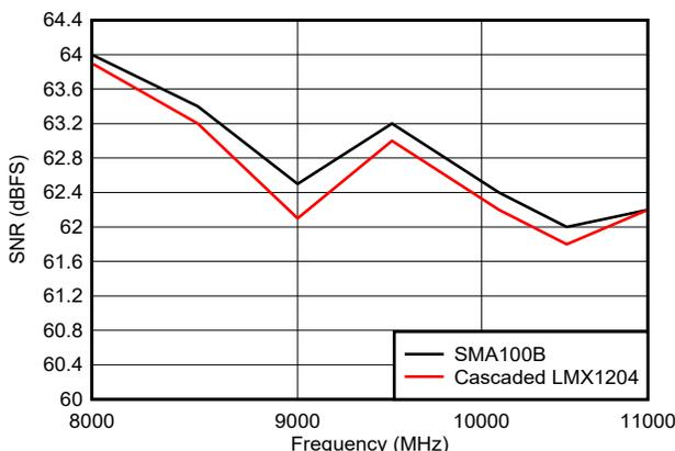
**Figure 2-9. AFE7950 - SNR vs. Clock Source vs. Frequency**
