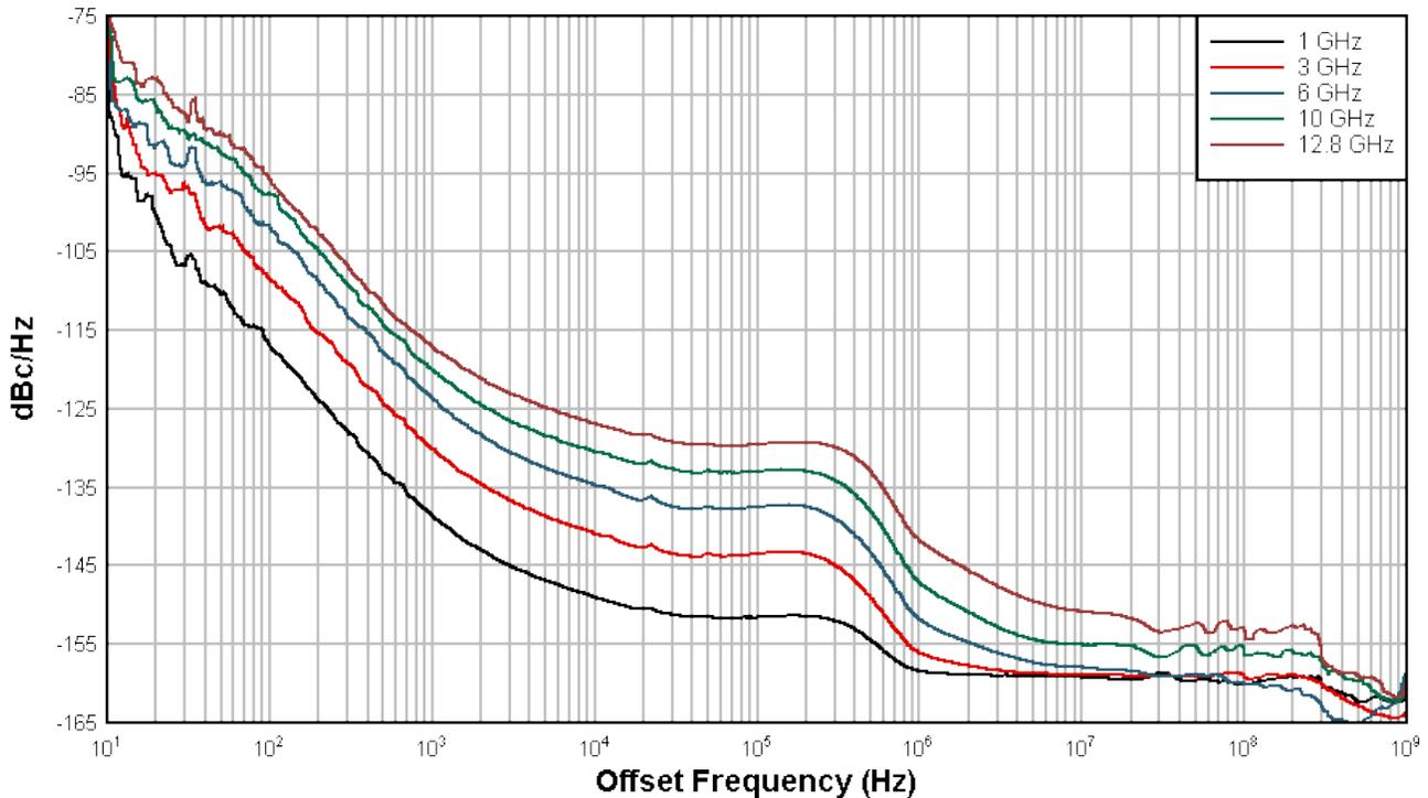
Figure 2-1. LMX1204EVM Phase Noise Measurements
