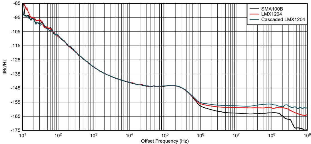
Figure 2-4. Phase Noise Comparison - 3 GHz
