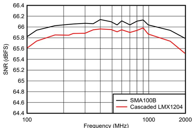
**Figure 2-8. ADC32RF54 - SNR vs. Clock Source vs. Frequency**
