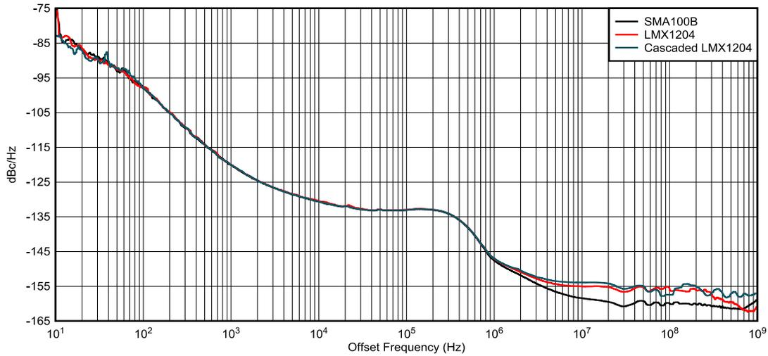
Figure 2-6. Phase Noise Comparison - 10 GHz
