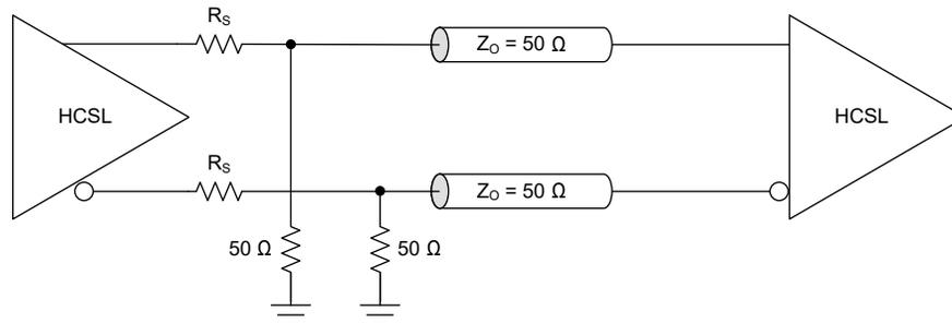
**Figure 4-1. HCSL Output Termination**
