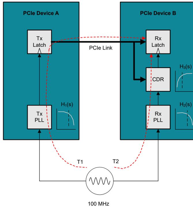
**Figure 3-4. REFCLK Common Clock Distribution**
