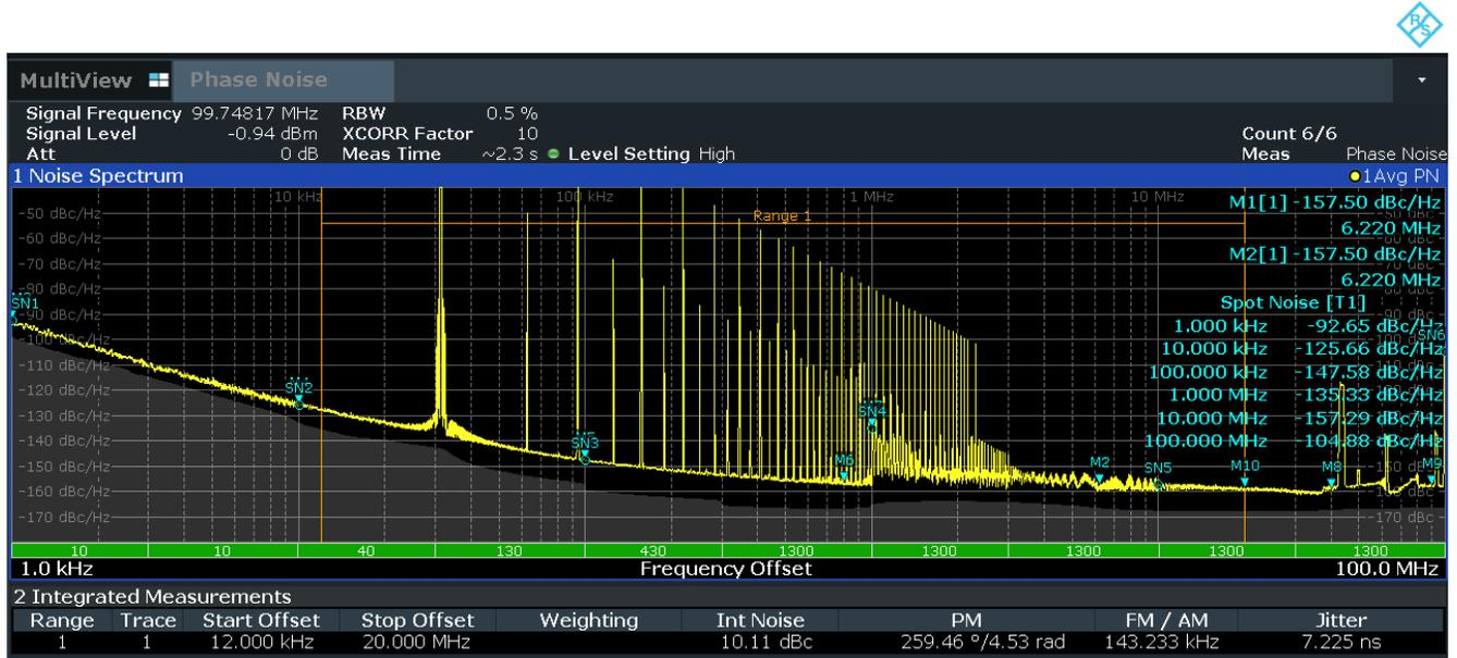
Figure 5-3. LMK3H0102 Phase Noise with SSC
