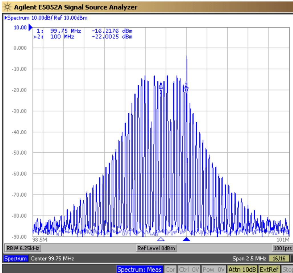
**Figure 3-3. 100 MHz REFCLK With No SSC and -0.5% Down-Spread SSC**
