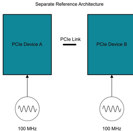
**Figure 3-2. Separate Reference Architecture**
