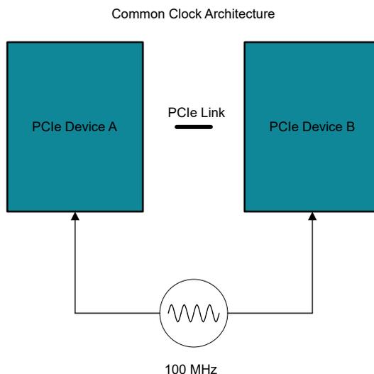
**Figure 3-1. Common Clock Architecture**
