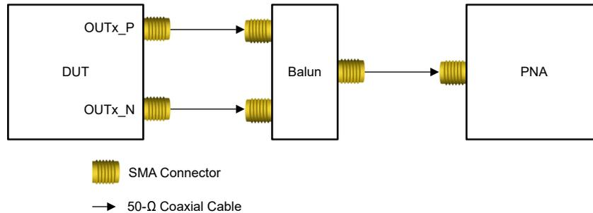
**Figure 5-1. PNA Measurement Test Setup**
