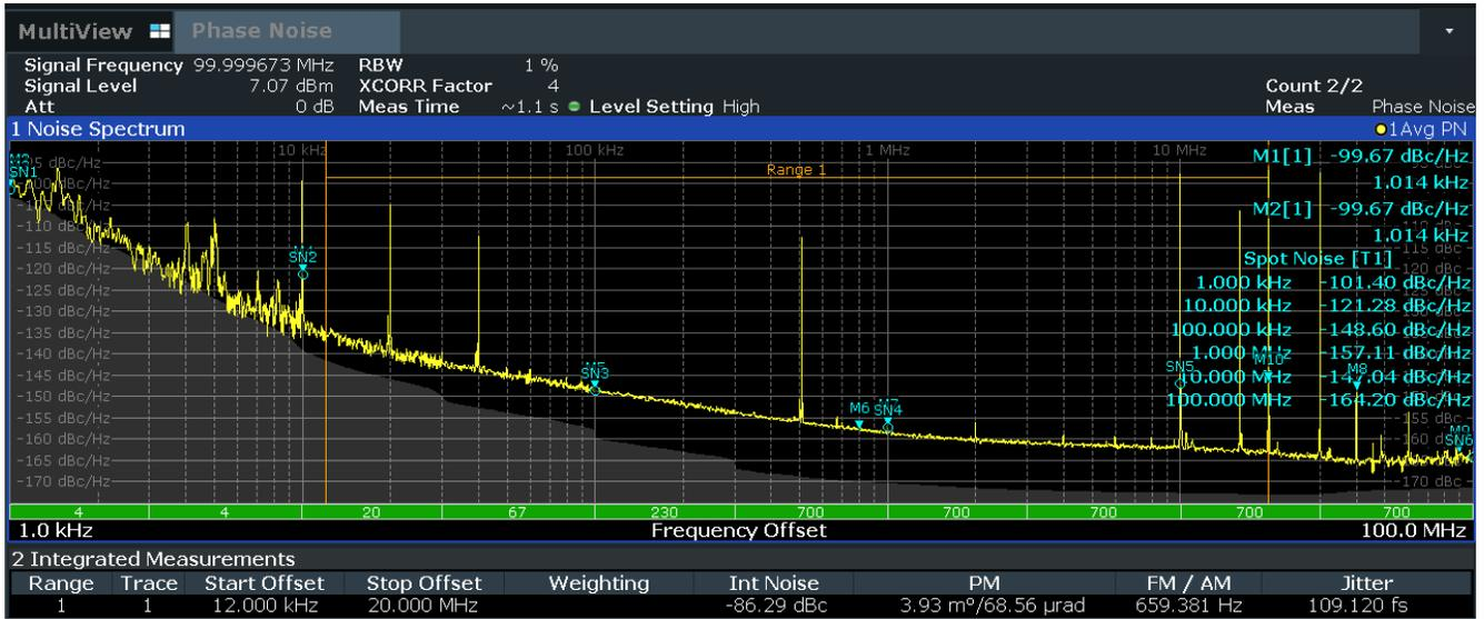
Figure 5-2. LMK3H102 Phase Noise Without SSC
