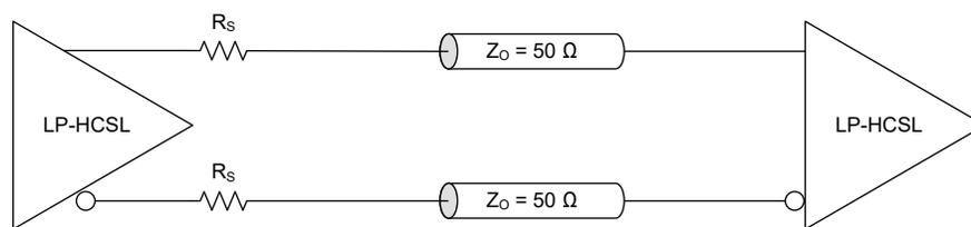
**Figure 4-2. LP-HCSL Output Termination**
