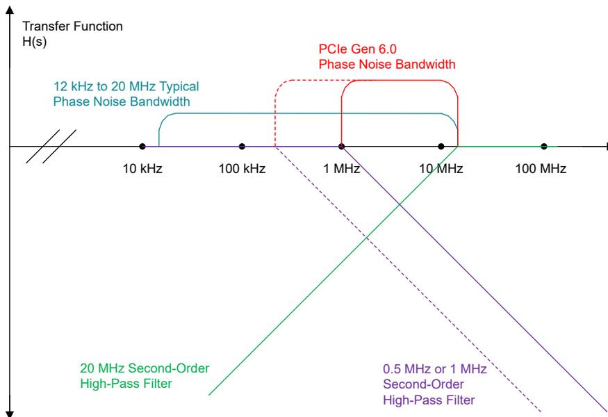
Figure 3-5. PCIe Bandwidth Visualization
