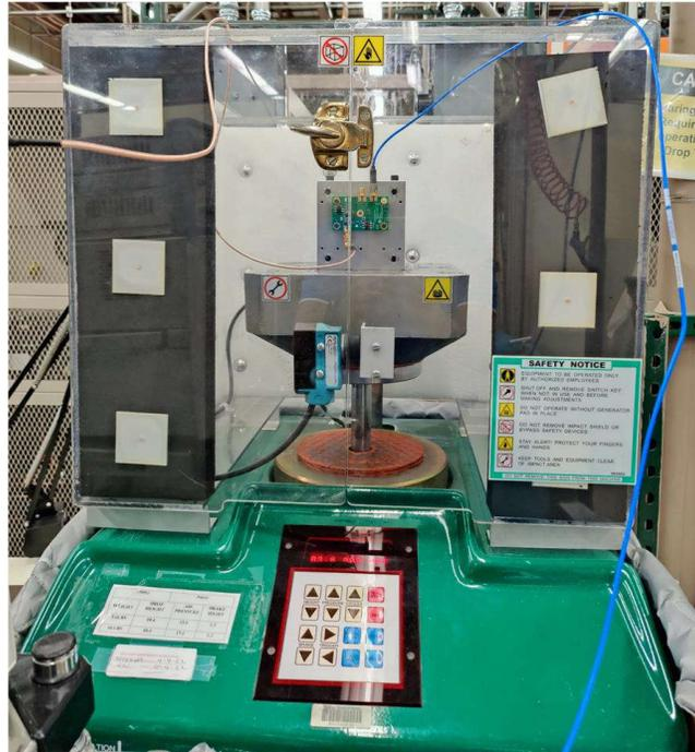
**Figure 3-19. Shock Test Setup**
