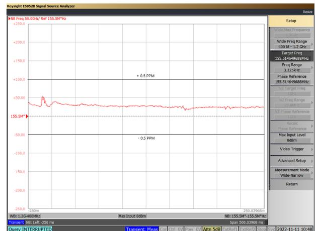
**Figure 3-27. Capture During Mechanical Shock Test of 6-pin DLF, Y axis**
