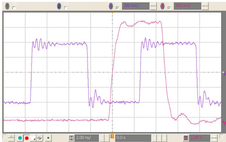
**Figure 3-16. Time-Critical SYNC Pulse**
