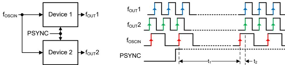
Figure 1-1. Phase Synchronization Concept
