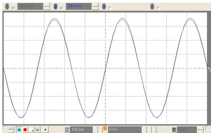
**Figure 3-9. After Phase Synchronization**
