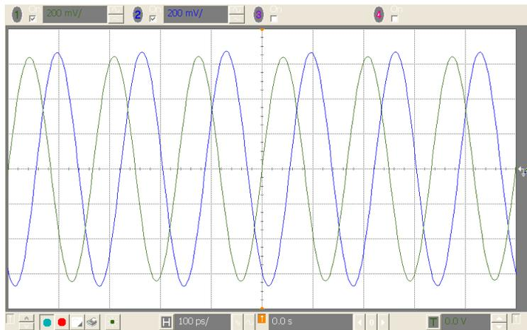
**Figure 3-15. Unable to SYNC With Non-Time Controlled SYNC Pulse**
