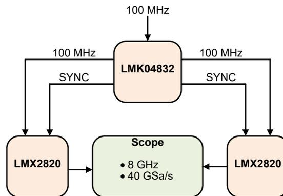
Figure 3-1. Test Setup
