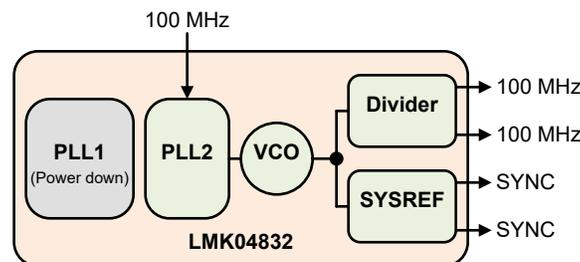
Figure 3-2. LMK04832 Configuration
