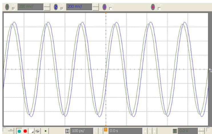
Figure 3-6. Phase Offset Due to Unsymmetrical Configuration
