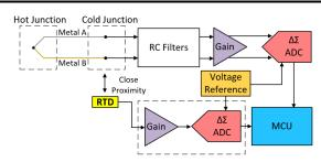
Figure 3. Cold Junction Compensation With RTD Block Diagram
