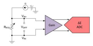
Figure 1. Simplified RTD Circuit
