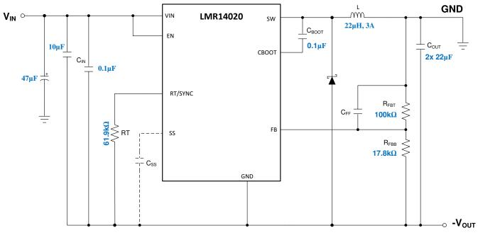
Figure 8-2. +5 V to -5 V, 1-A Design with the LMR14020
