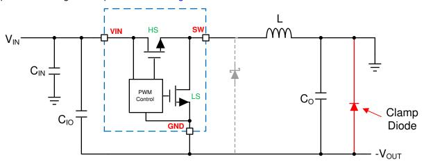
Figure 7-4. Output Clamp Diode
