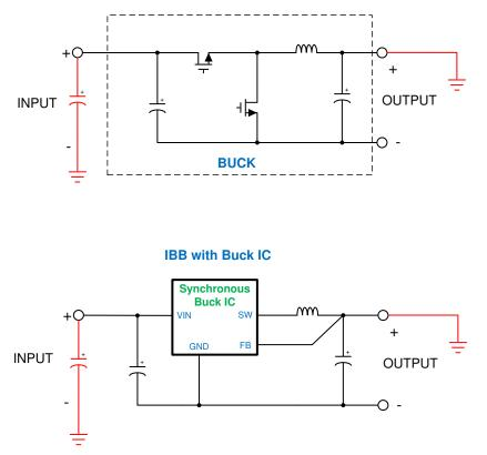
Figure 2-2. Converting a Buck to an Inverting Buck-Boost
