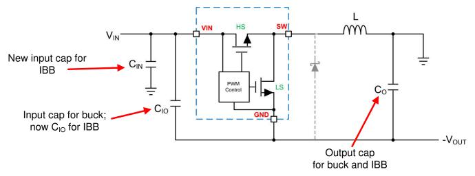
Figure 5-1. IBB External Components
