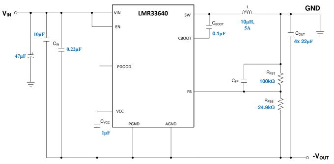
Figure 8-1. +12 V to -5 V, 3-A Design with the LMR33640
