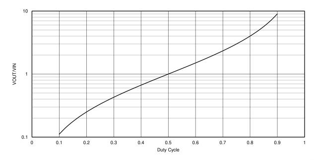
Figure 3-2. Conversion Ratio vs Duty Cycle
