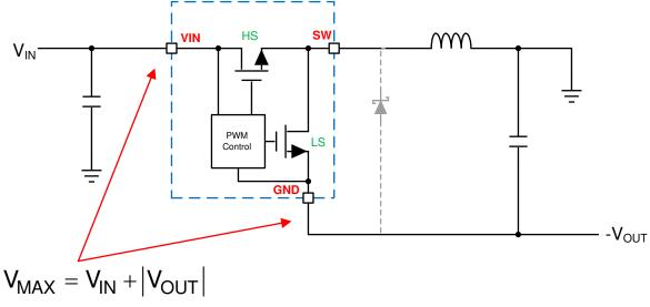
Figure 4-1. Voltage Stress on an IBB
