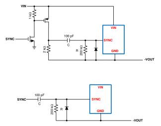
Figure 7-2. Synchronization Level Shifters
