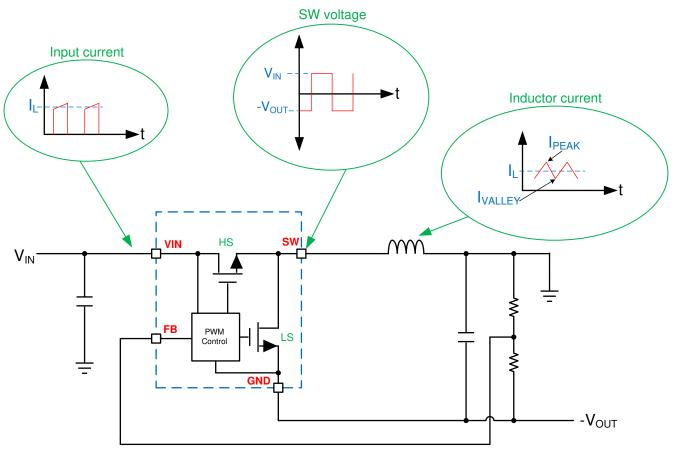
Figure 3-1. Inverting Buck-Boost Waveforms
