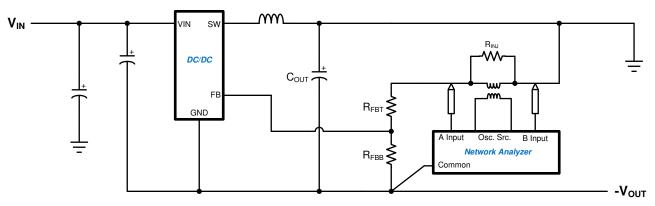
Figure 4-2. Set-up for Measuring Bode Plots for an IBB
