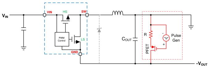
Figure 4-3. Set-up for Measuring Load Transient Response for an IBB
