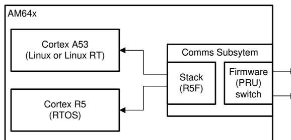
**Figure 1-2. Implementation Using the Integrated Industrial Communication Stack**
