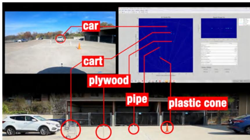
**Figure 6.** Multiple types of objects detected by a mmWave radar sensor.
