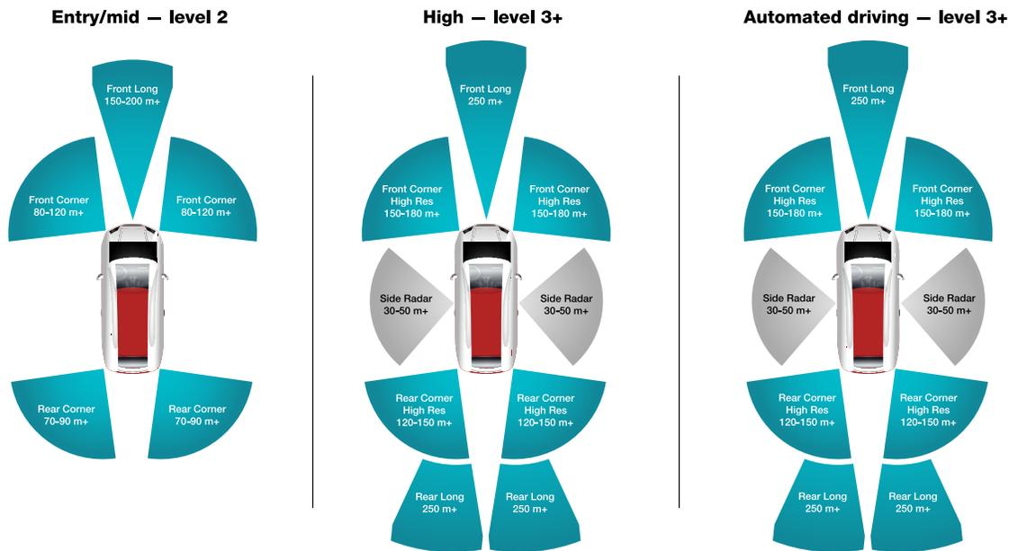
**Figure 1.** Radar sensors enable advanced levels of autonomy.
