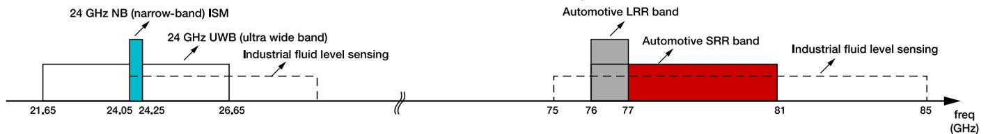
**Figure 2.** 77-GHz Wide bandwidth with provides higher range resolution and accuracy.
