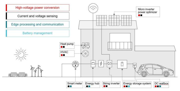
Figure 1. A Residential Solar Energy Generation and Energy Storage System Installation
