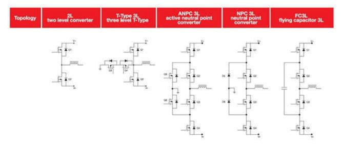
Figure 3. Power Topologies for Half-bridge and Branch Equivalent
