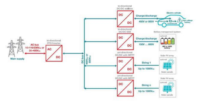
Figure 2. A Typical Solar Inverter System With an Energy Storage System
