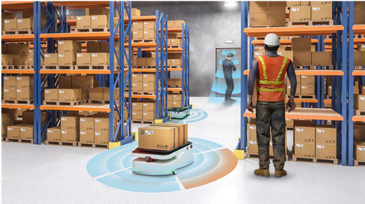
**Figure 2. A Warehouse Robot Uses Radar Sensing.**
