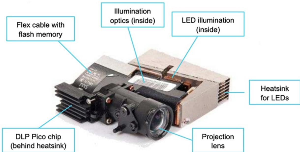
Figure 1. Example Optical Module
