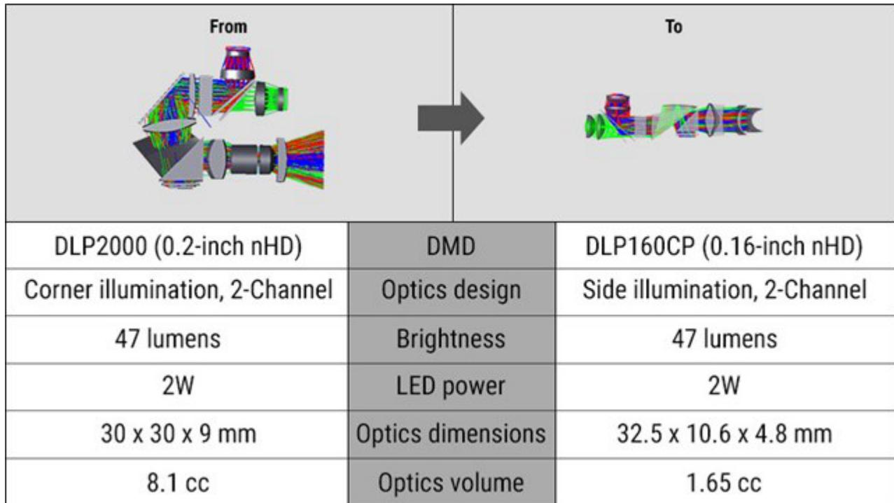
**Figure 3. Optical Module Comparison**
