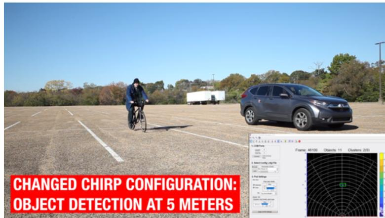
**Figure 6. Detection of a Cyclist at 5 M Using the Door Obstacle Detection Sensor**
