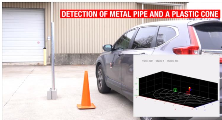
**Figure 3. Detection of a Plastic Cone (Placed inside the Collision Zone) and Metal Pole (Placed outside the Collision Zone)**
