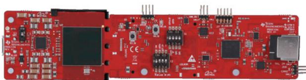
Figure 2. A TI Radar Sensor with AoP Technology
