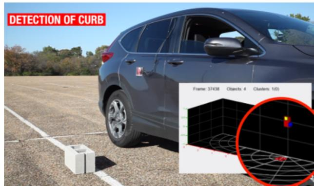
**Figure 4. Detection of a Low-height Curb Using TI's AWR1843AOP EVM**
