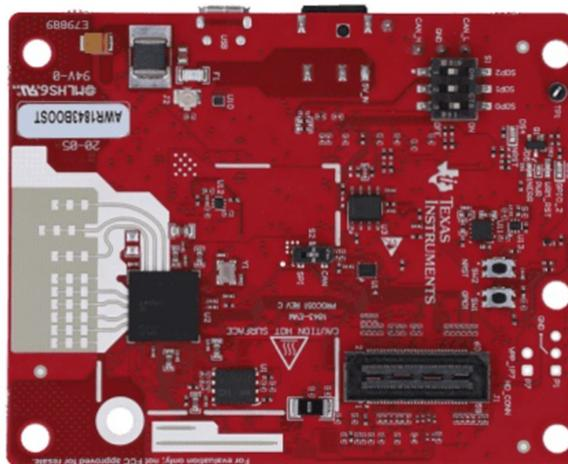
Figure 1. A Radar Sensor with an Antenna on the PCB
