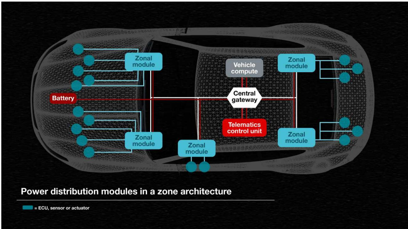
**Figure 3. Power distribution modules in a zone architecture**
