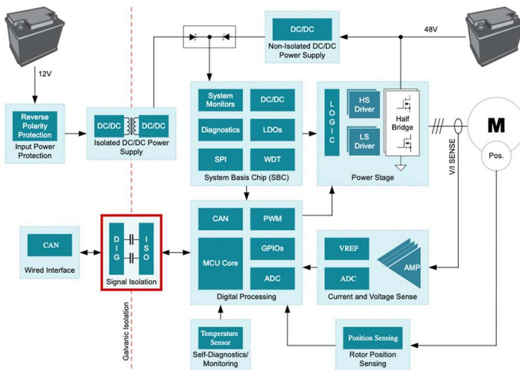
**Figure 1. Digital isolator protecting the low-voltage side of a 48-V starter/generator system**
