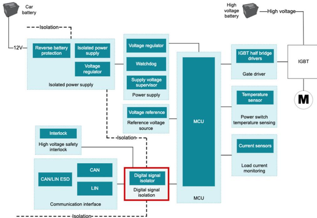
**Figure 2. Digital isolator protecting the low-voltage side of a 48-V HVAC compressor module**
