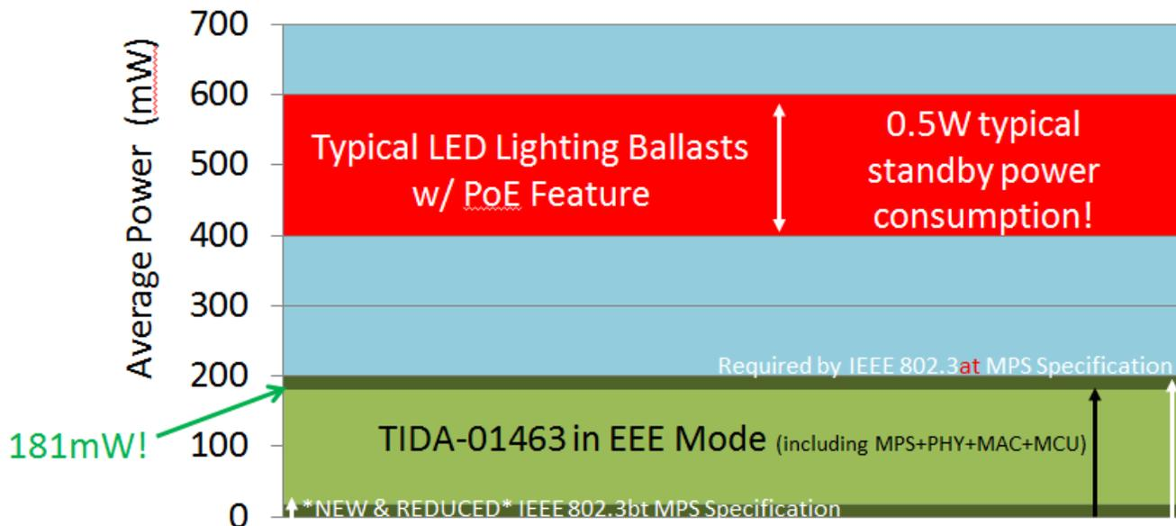
**Figure 1. Input Power Consumption in Standby (Lights off)**
