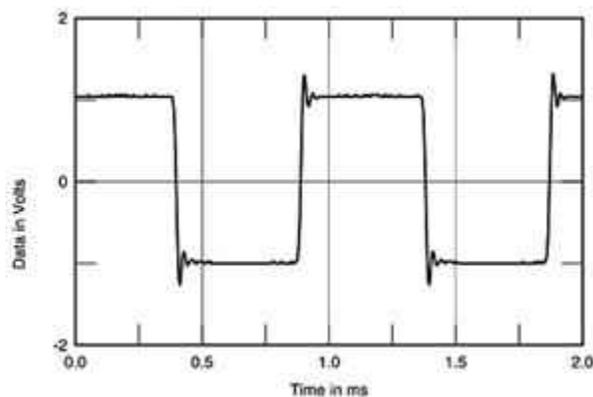
**Figure 4. Example PFC Controller Output Waveform**
