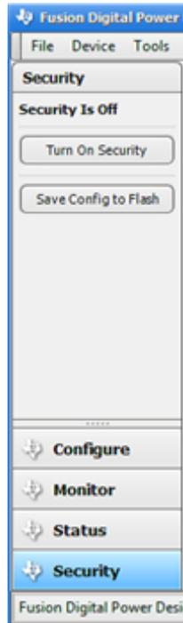
**Figure 4. Enabling the Security Feature in the Fusion Digital Power Designer GUI**
