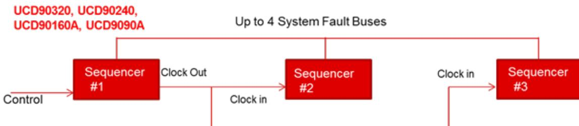
**Figure 5. Cascading Multiple UCD90xxx Devices**
