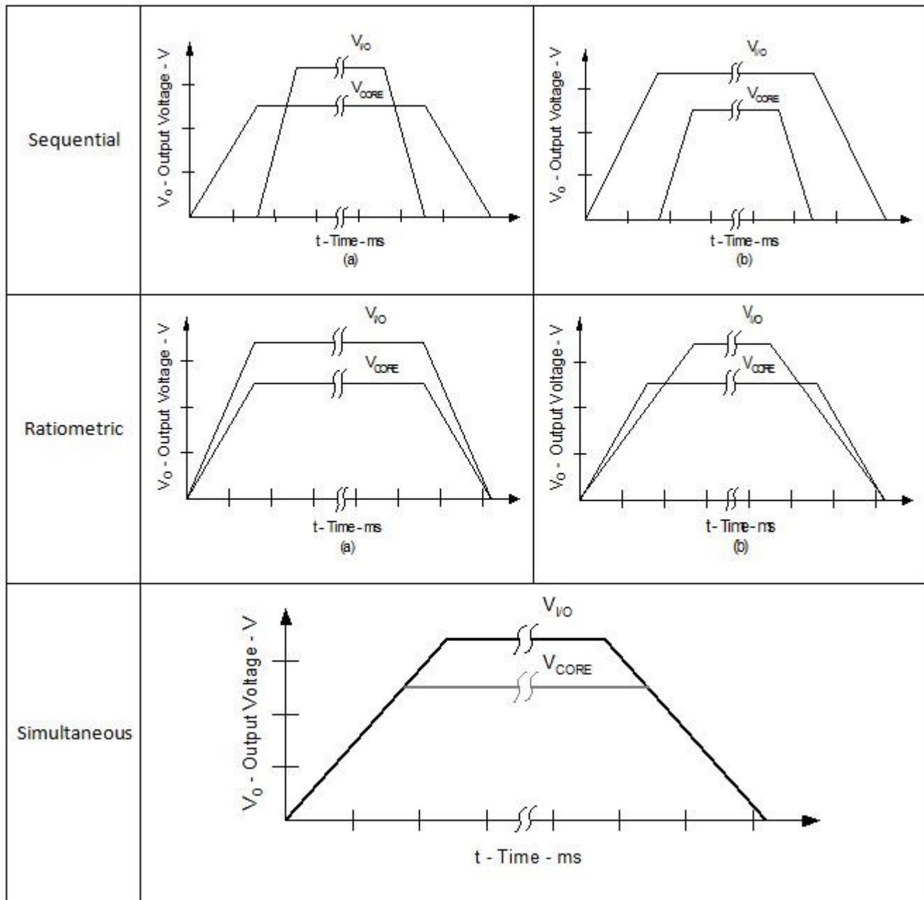
Figure 3. Sequencing Schemes for Multiple Voltage Rails
