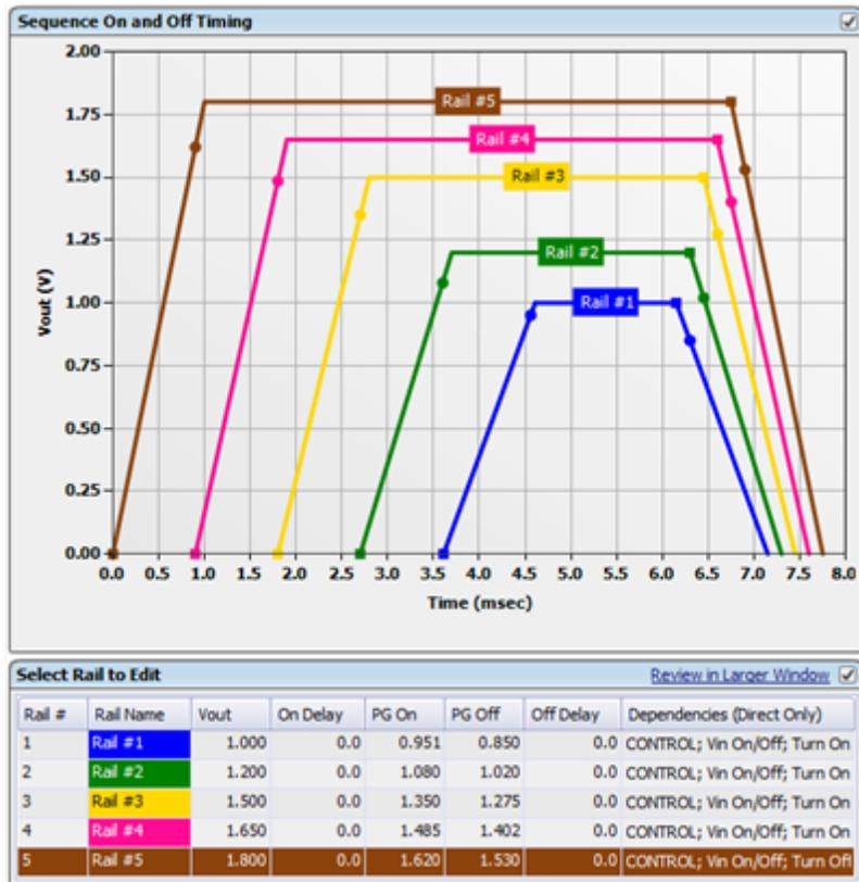
**Figure 2. Sequence on and off Timing Window (Rail Config)**
