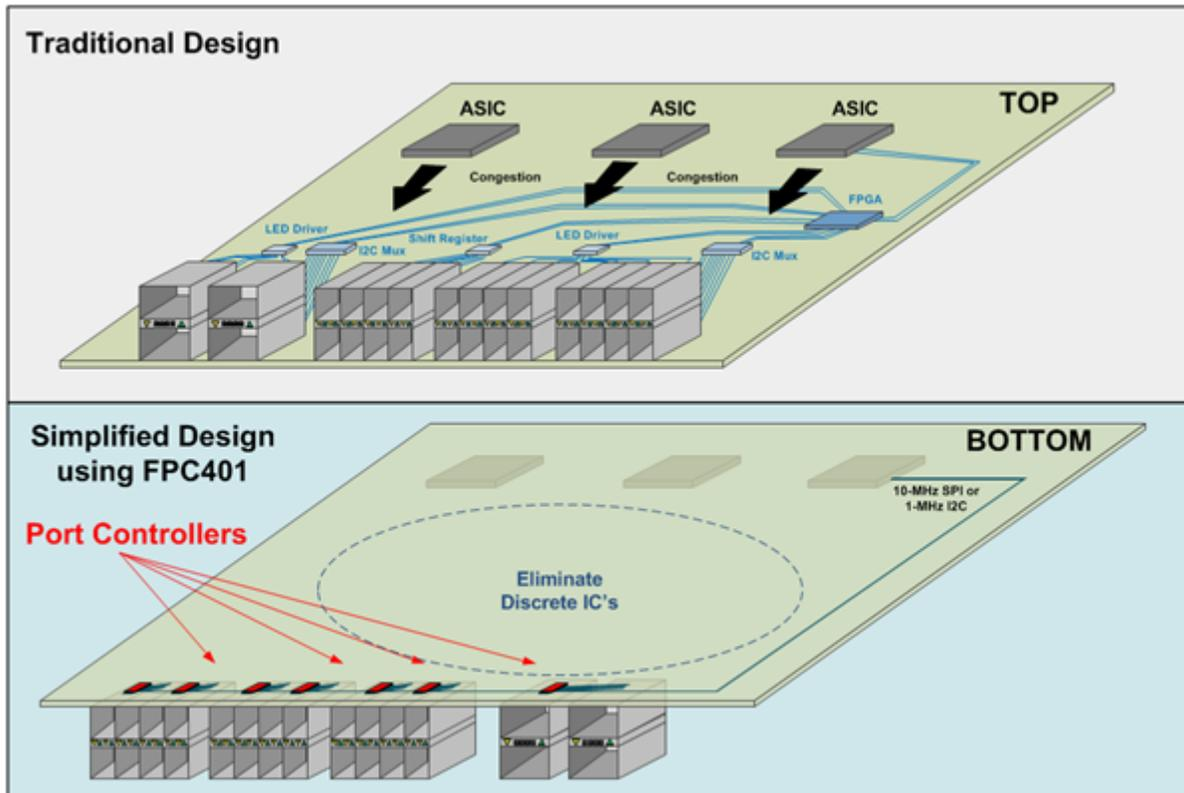
Figure 1. A traditional solution vs. an FPC401-based solution
