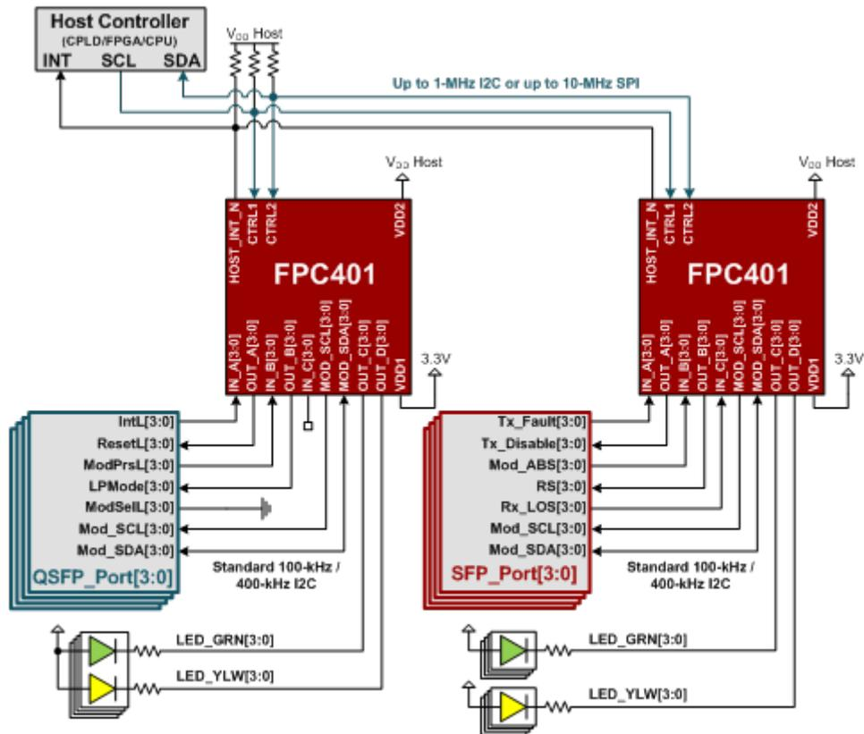
**Figure 2. FPC401 simplified schematic for a typical application**
