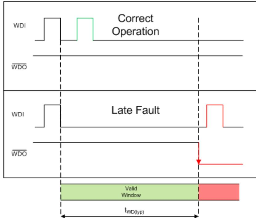
**Figure 2. Operation of a Standard Watchdog Timer**
