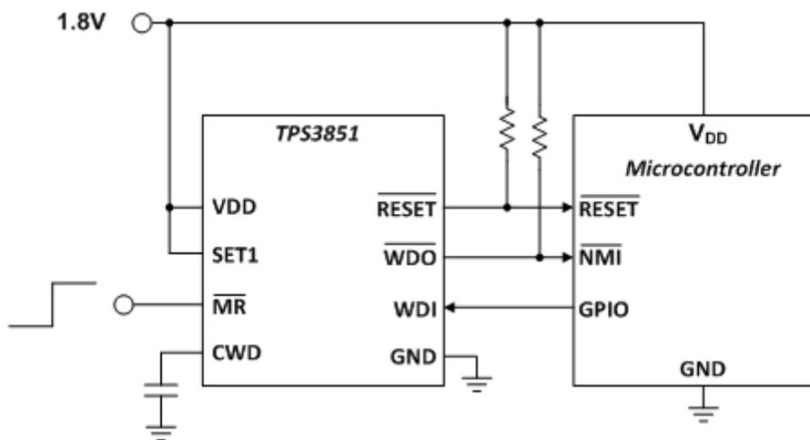
Figure 1. Watchdog Monitoring Provided by the [TPS3851](#)
