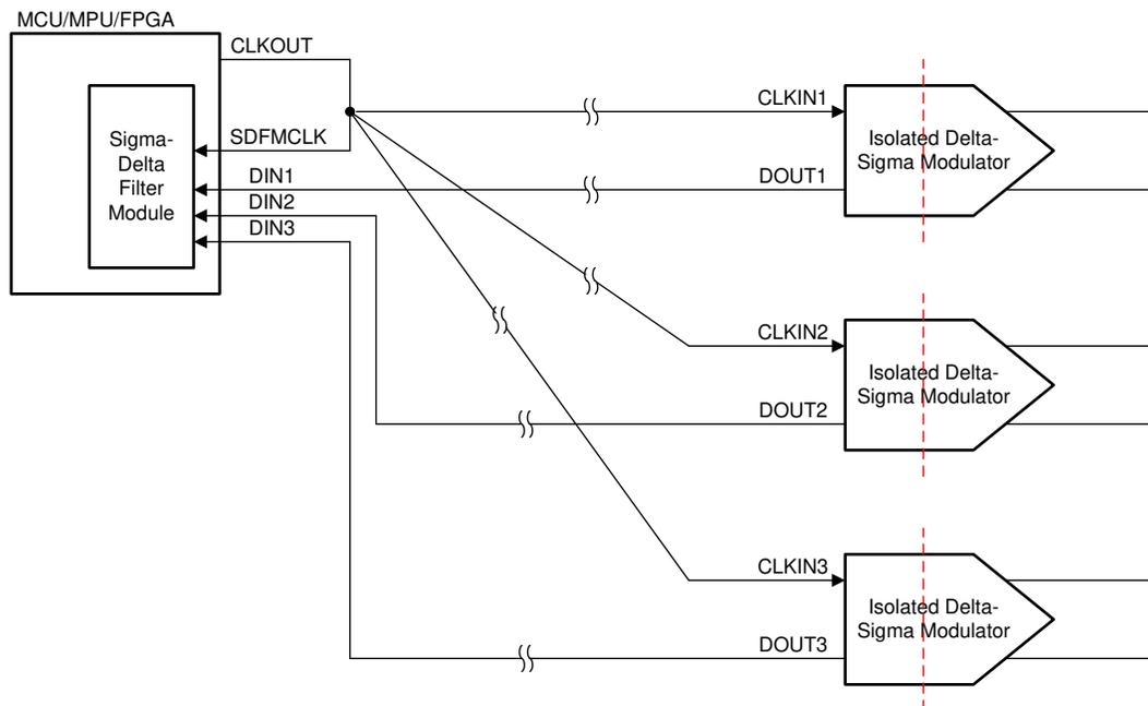
**Figure 3. Star Clock Routing**
