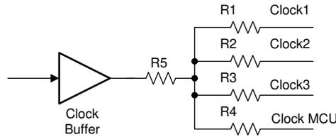
**Figure 18. Series Termination Configuration**
