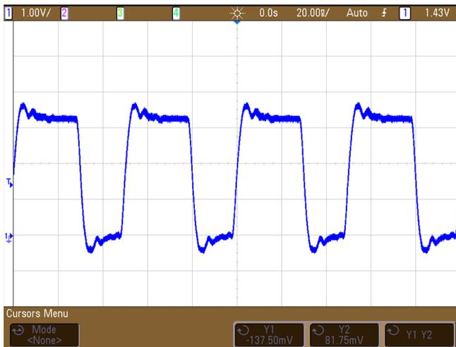
Figure 14. Clock Signal Probed At Buffer Output - No Termination
