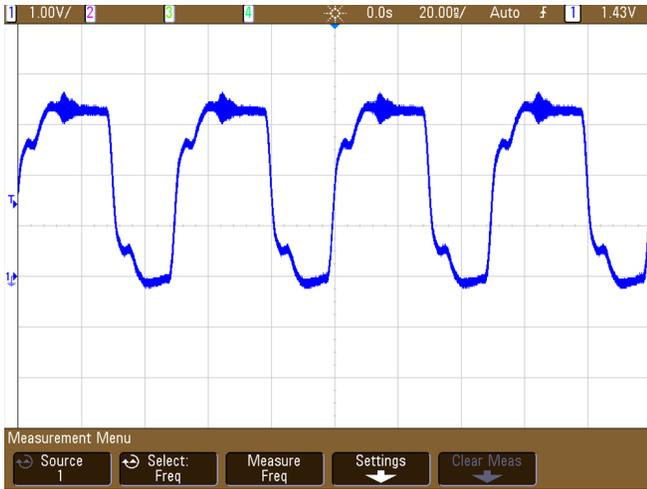
Figure 42. Clock Signal Probed At Buffer Output - Individual Series Termination
