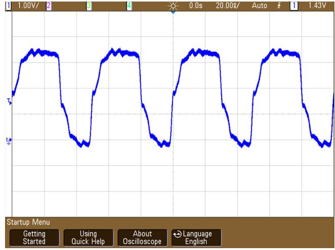
**Figure 37. Clock Signal Probed At Modulator 3 - Thevenin AC Termination**
