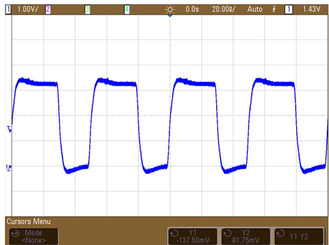
Figure 26. Clock Signal Probed At Modulator 1 - Individual Series Termination
