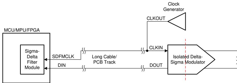
Figure 48. MCU to Modulator Interface - Clock Generated by External IC
