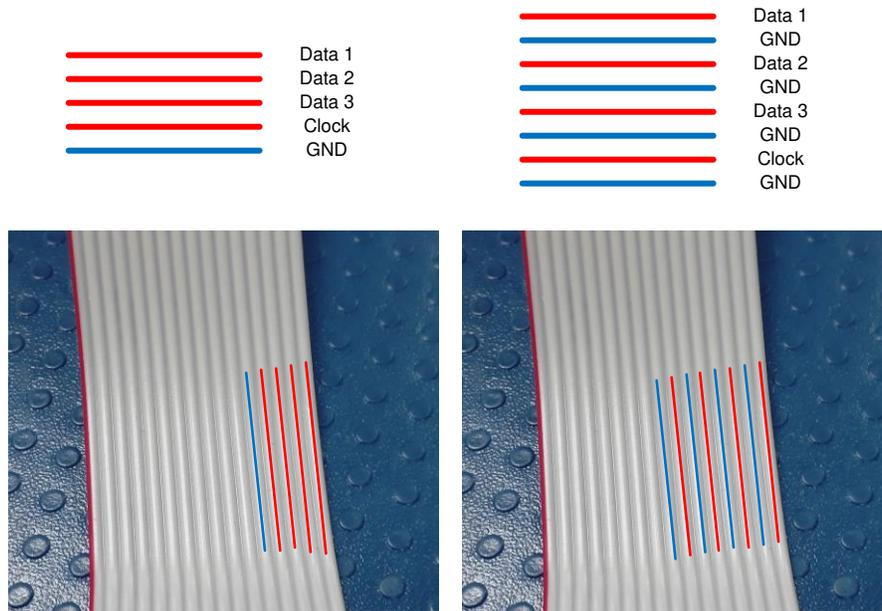
**Figure 33. Ground Signal Routing in Flat Cables**
