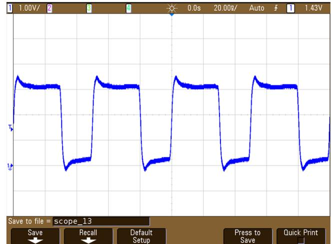
Figure 12. Clock Signal Probed at Modulator 3 - Thevenin AC Termination
