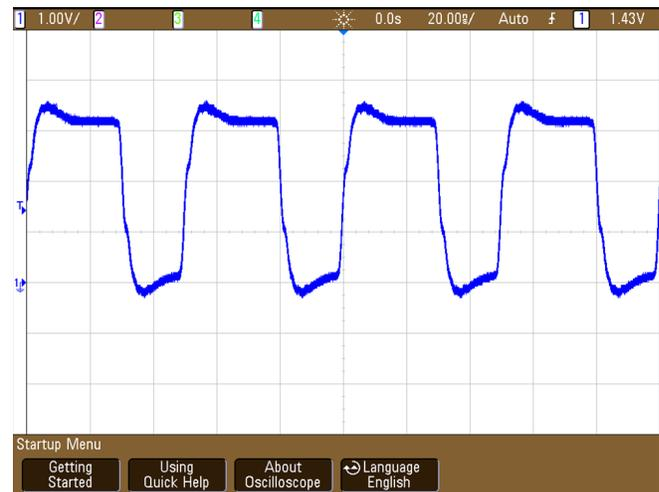
**Figure 35. Clock Signal Probed At Modulator 3 - Thevenin AC Termination**
