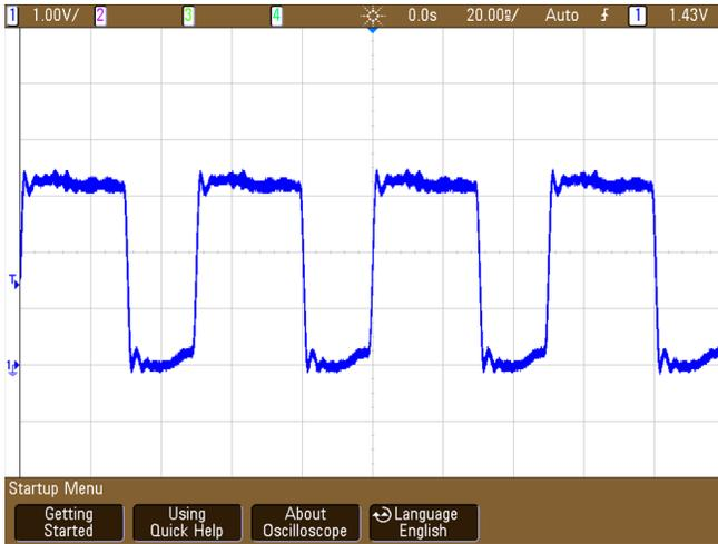
Figure 29. Clock Signal Probed At Buffer Output - No Termination
