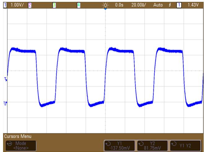
Figure 24. Clock Signal Probed At Modulator 3 - Individual Series Termination
