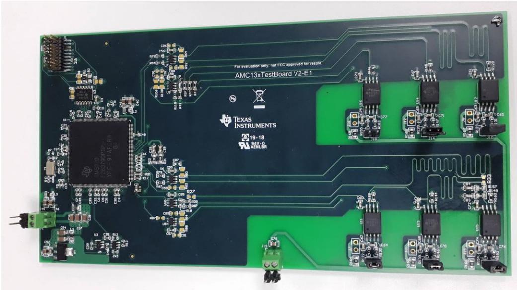
**Figure 27. Test Board With no Connector and Cables**
