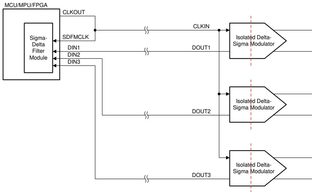
**Figure 2. Daisy-Chain Clock Routing**
