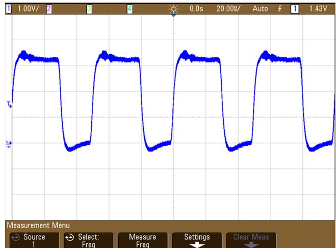
**Figure 41. Clock Signal Probed At Modulator 1 - Individual Series Termination**
