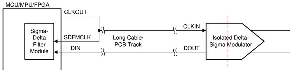
**Figure 46. MCU To Modulator Interface - Clock Generated By MCU**
