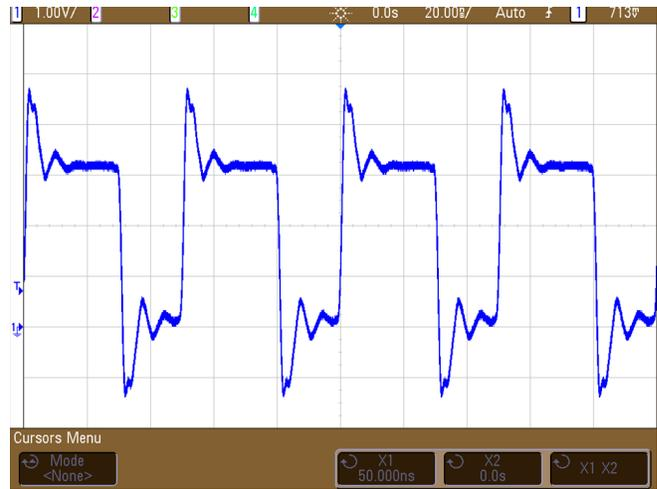
Figure 6. Clock Signal Probed at Modulator 3 - No Termination
