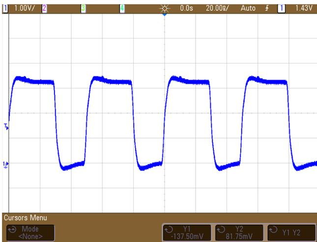
Figure 25. Clock Signal Probed At Modulator 2 - Individual Series Termination
