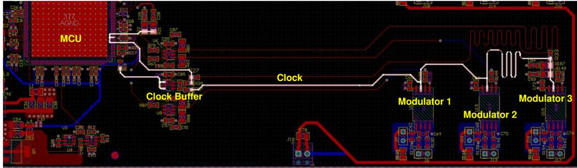
Figure 4. Daisy-Chain Routing Example
