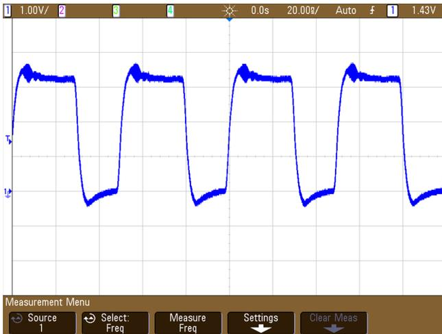
**Figure 40. Clock Signal Probed At Modulator 2 - Individual Series Termination**
