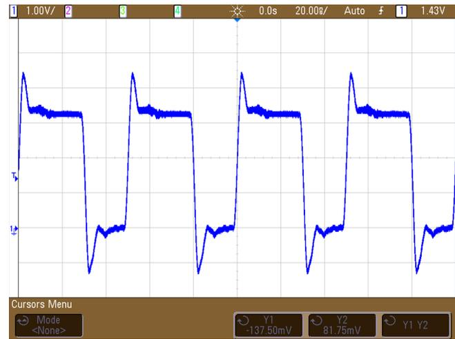
Figure 15. Clock Signal Probed At Modulator 3 - No Termination
