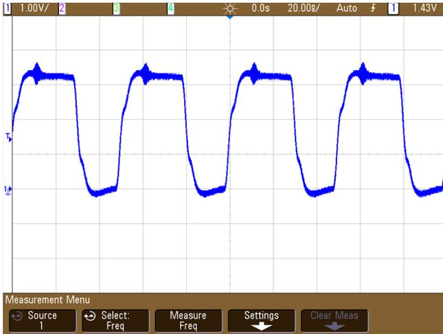
**Figure 38. Clock Signal Probed At Buffer Output - Individual Series Termination**
