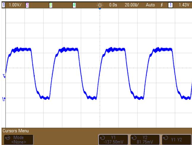
**Figure 19. Clock Signal Probed At Buffer Output - Single Series Termination**
