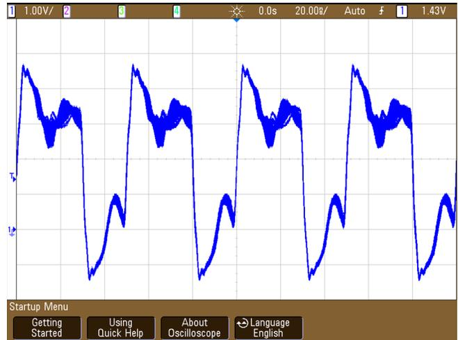
Figure 30. Clock Signal Probed At Modulator 3 - No Termination
