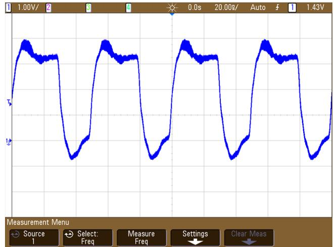
Figure 43. Clock Signal Probed At Modulator 3 - Individual Series Termination
