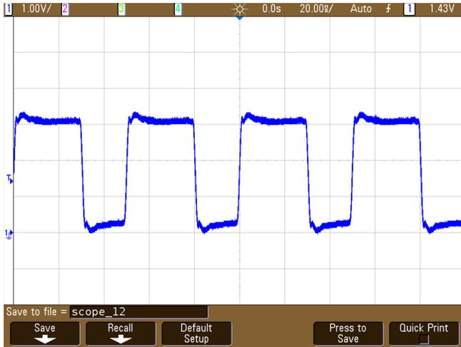
Figure 11. Clock Signal Probed at Buffer Output - Thevenin AC Termination
