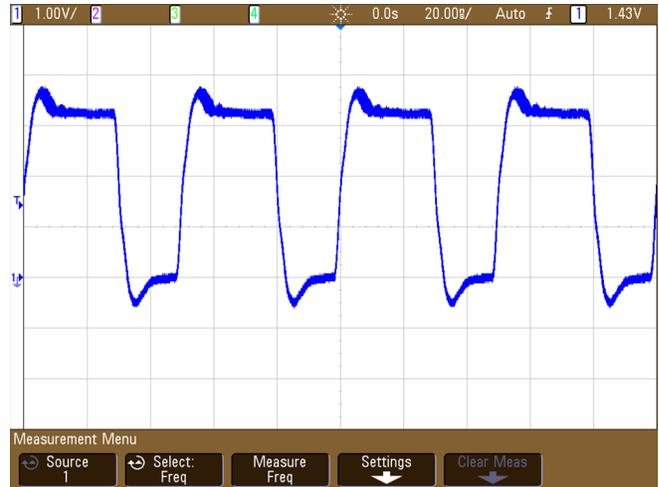
**Figure 39. Clock Signal Probed At Modulator 3 - Individual Series Termination**
