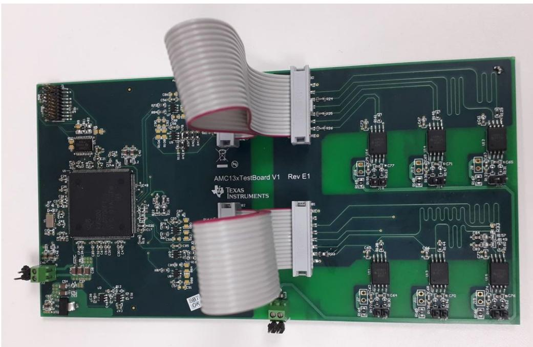
**Figure 28. Test Board Modified With Intermediate Connector and Flat Ribbon Cables**
