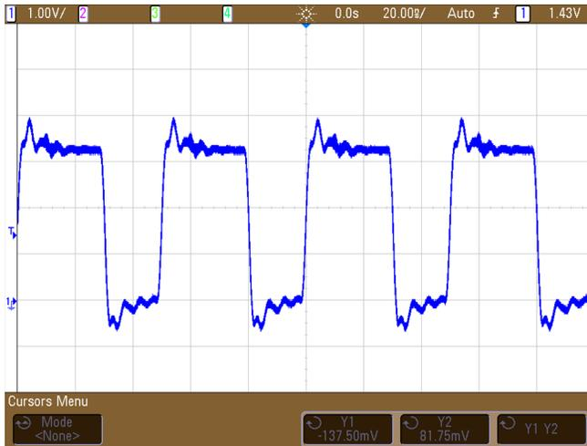
**Figure 16. Clock Signal Probed At Modulator 2 - No Termination**
