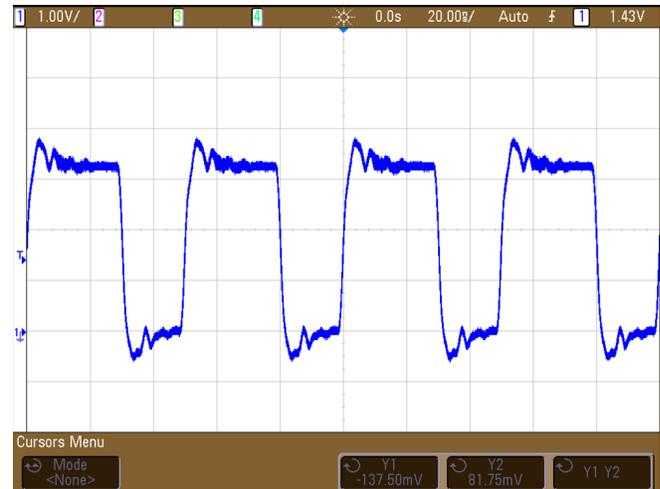
**Figure 17. Clock Signal Probed At Modulator 1 - No Termination**
