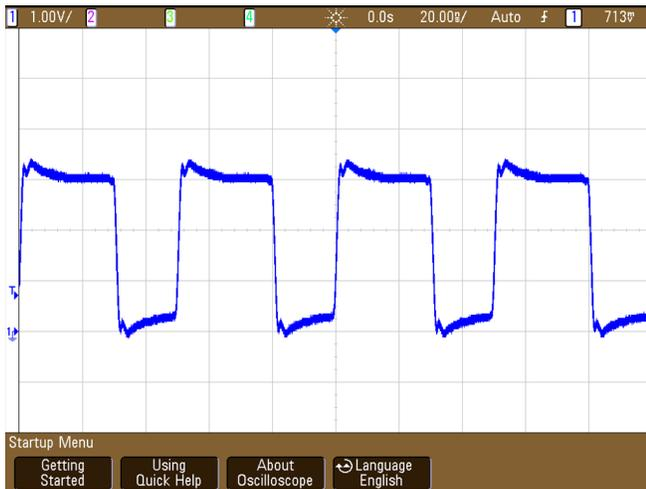
**Figure 8. Clock Signal Probed at Buffer Output - Thevenin Termination**
