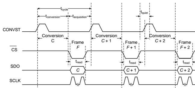
**Figure 2. Standard 3-wire SPI Interface with ADS8920B**
