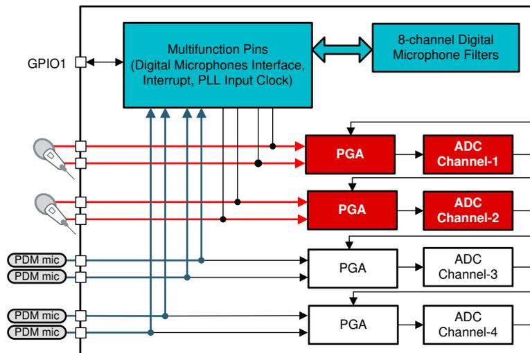
Figure 11. Combination Microphones System Block Diagram
