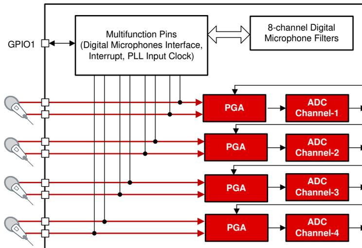
Figure 9. Analog Microphones System Block Diagram
