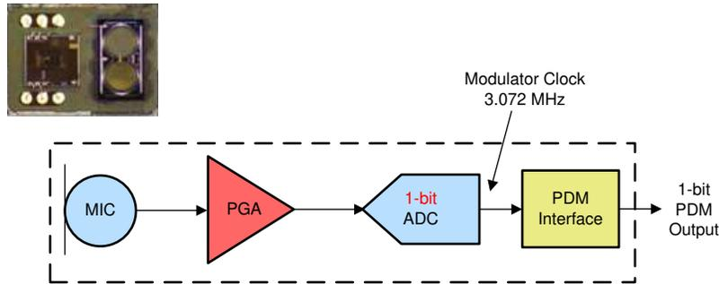
Figure 2. Digital PDM Microphone for 1-bit Output
