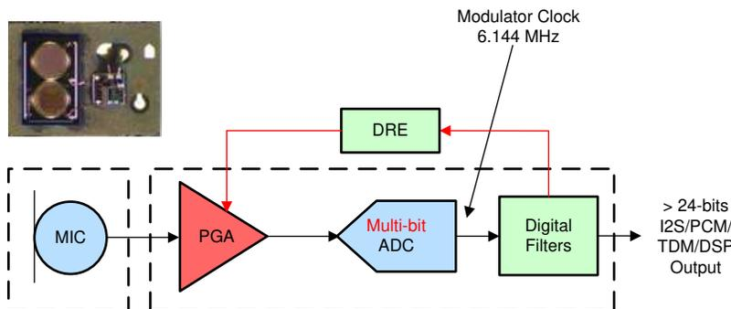
Figure 3. Analog Microphone with ADC for Multi-bit Output
