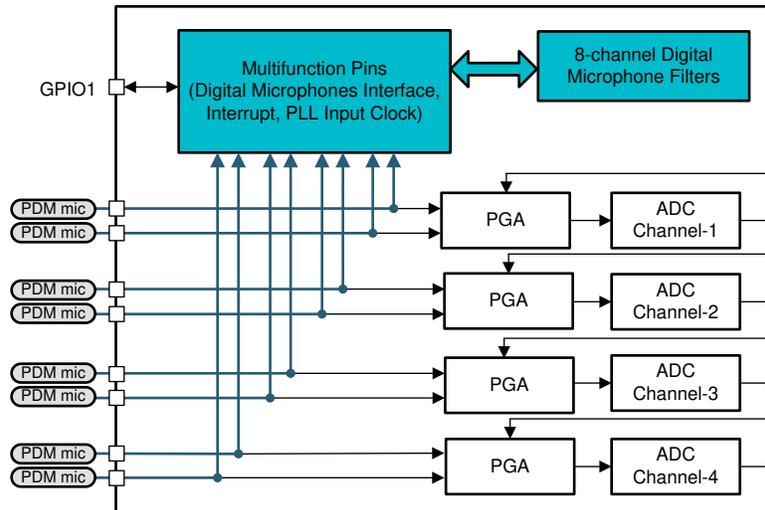
Figure 10. Digital PDM Microphones System Block Diagram
