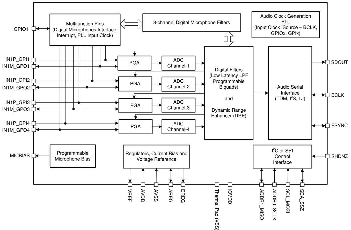
Figure 8. Internal Block Diagram of the TLV320ADC5140
