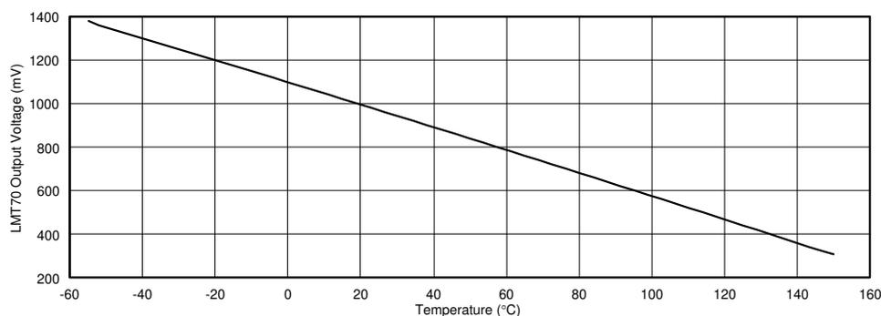
Despite the appearance, the LMT70 output transfer function is not linear. Accurately determining the temperature requires interpolation from a lookup table or calculation from a polynomial equation.
