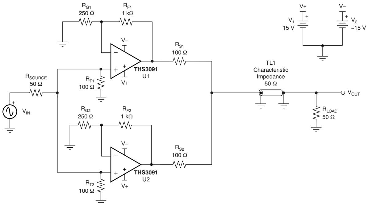
**Figure 3. Two THS3091 Amplifiers in Load Sharing Configuration**
