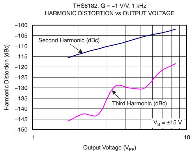
**Figure 1. 1-kHz Harmonic Distortion vs. Output Voltage (THS6182)**
