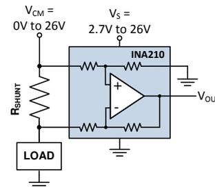
Figure 2. INA210: Current Sensing Amplifier
