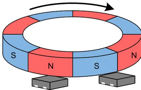
**Figure 4. Magnetic Incremental Encoder**
