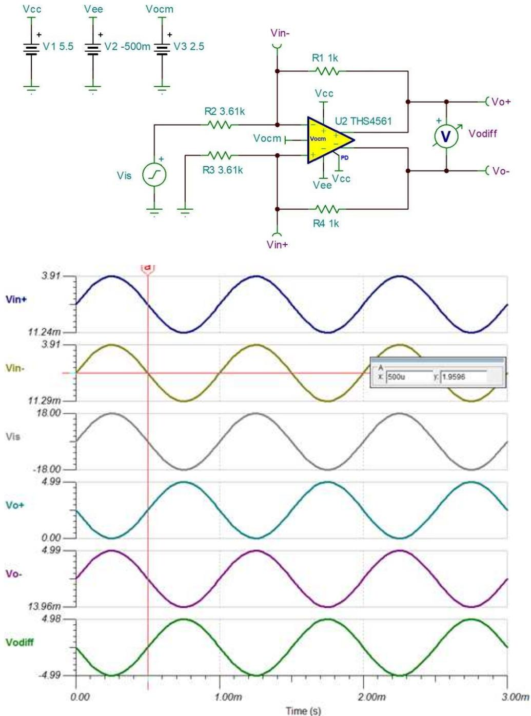
Figure 6. THS4561 TINA Circuit and Simulated Results
