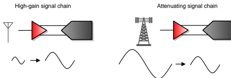
**Figure 1. High Gain versus Attenuating Signal Chains**
