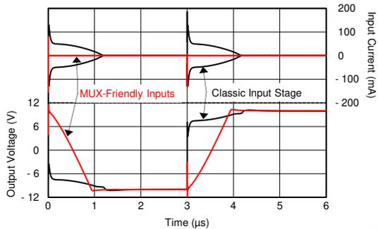
**Figure 3. Switching Timing Diagram**
