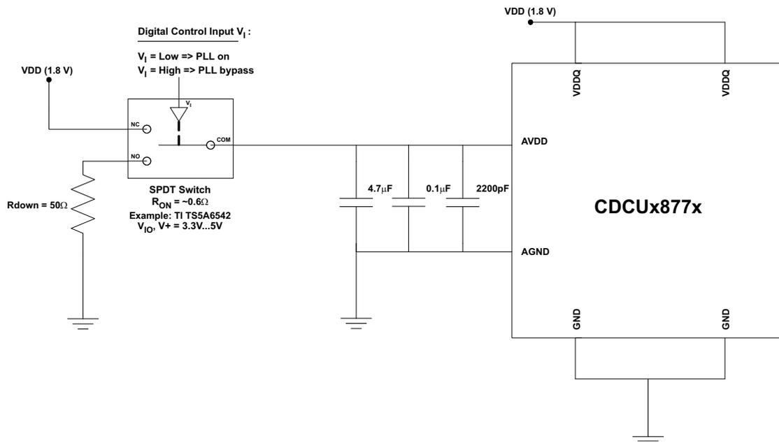
Figure 3. Example Circuit for Switching PLL Into Bypass Mode
