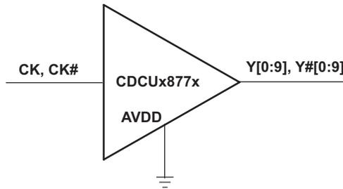
Figure 2. The CDCUx877x Used as 1:10 Clock Buffer
