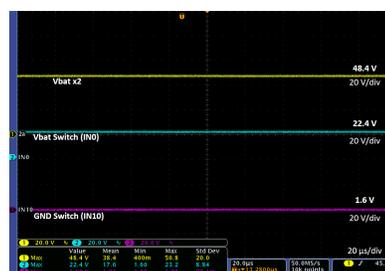
Figure 3. Double Battery Condition, Switches Connected
