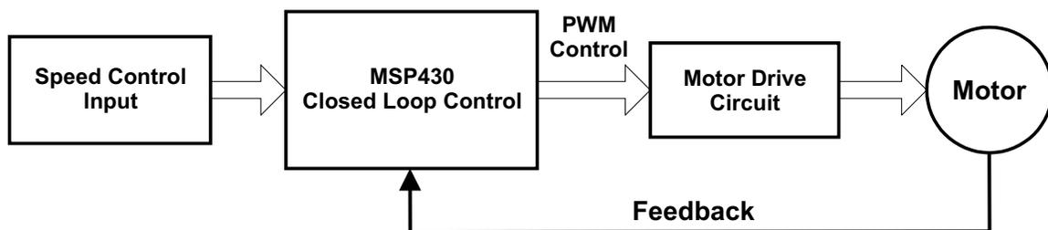
Figure 6. Closed-Loop Control – Basic Block Diagram
