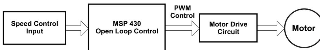
**Figure 1. Open-Loop Control – Basic Block Diagram**
