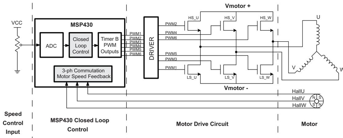
**Figure 7. Closed-Loop Control – MSP430 Based Implementation**
