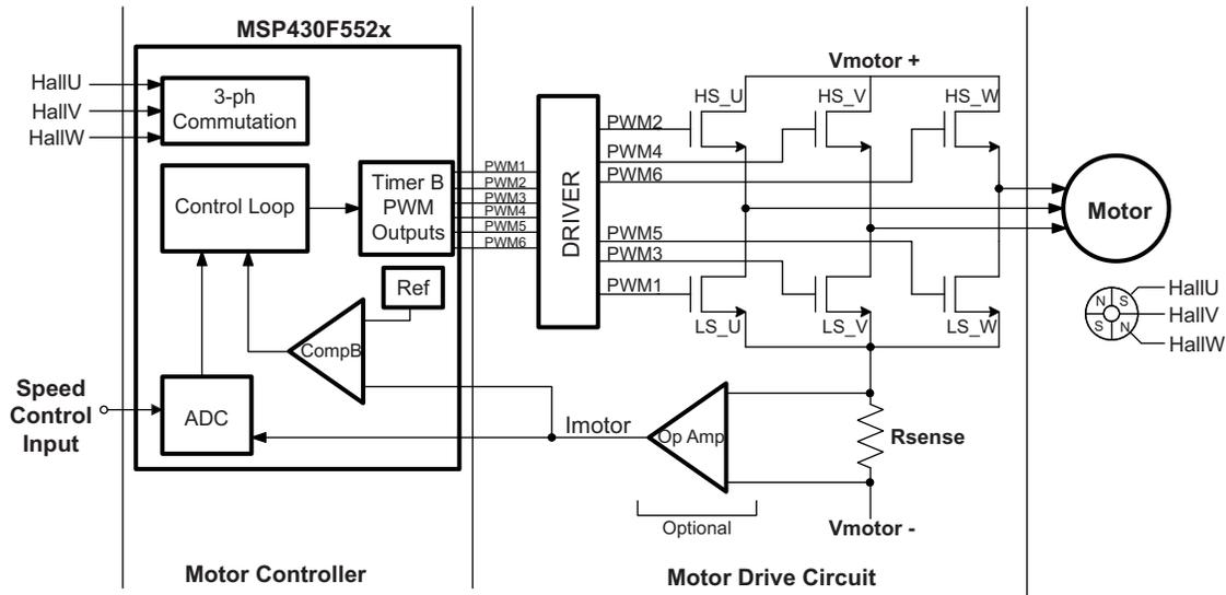
Figure 11. Current Monitor and Overcurrent Protection Circuitry
