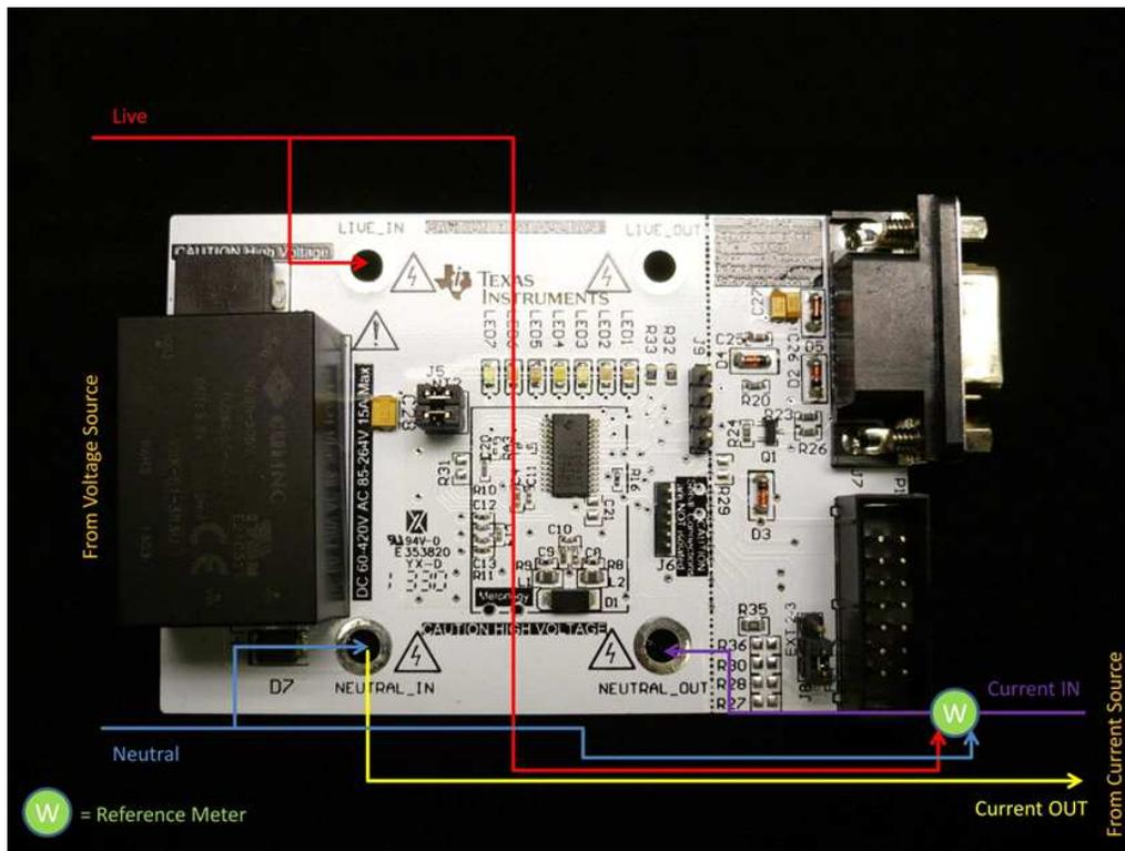
Figure 9. Calibration Setup
