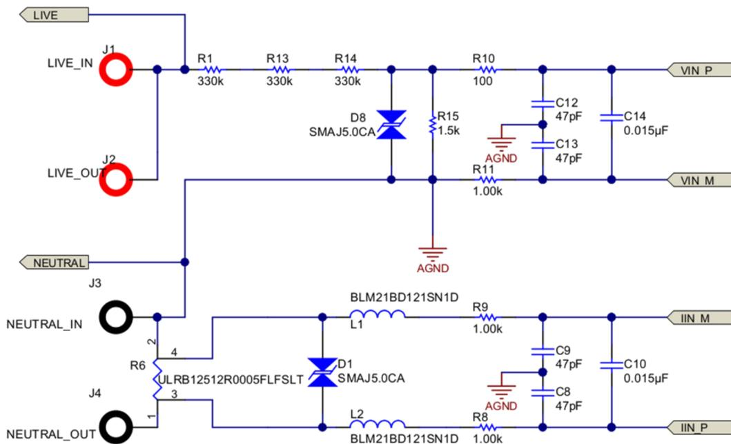
Figure 2. Voltage and Current Sensor Interface Circuit
