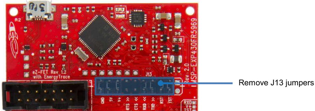
**Figure 3. Remove J13 Jumpers Before Starting ULPBench**
