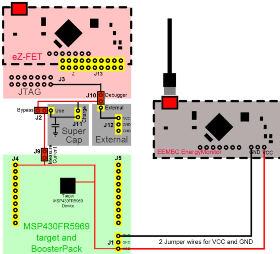
Figure 4. VCC and GND Connection
