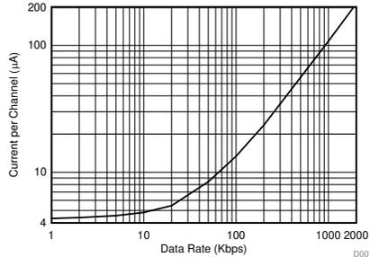
**Figure 4. ISO7041 Individual Channel Power Versus Data Rate**
