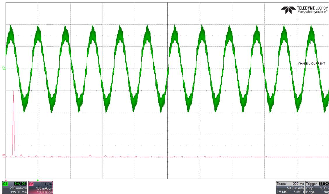
**Figure 2-5. Phase current waveform and FFT - Dead time compensation enabled**
