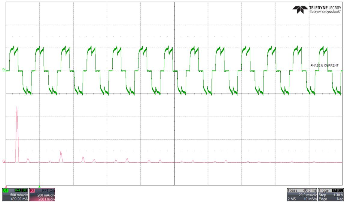
Figure 2-7. Phase current waveform and FFT - 120° Trapezoidal commutation
