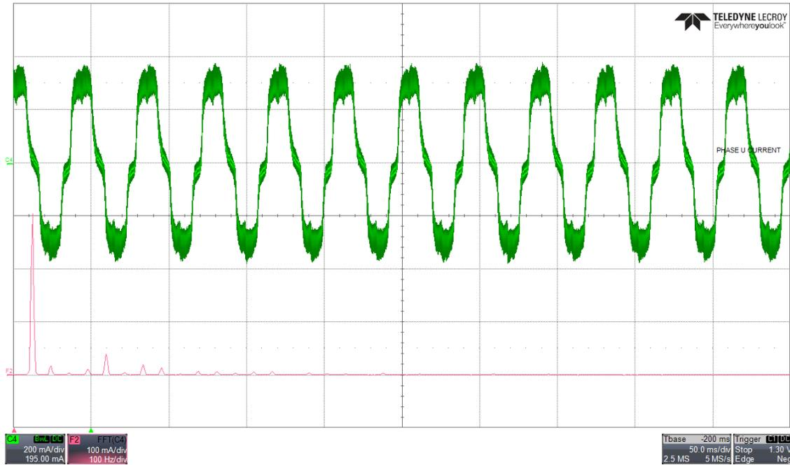
**Figure 2-4. Phase current waveform and FFT - Dead time compensation disabled**
