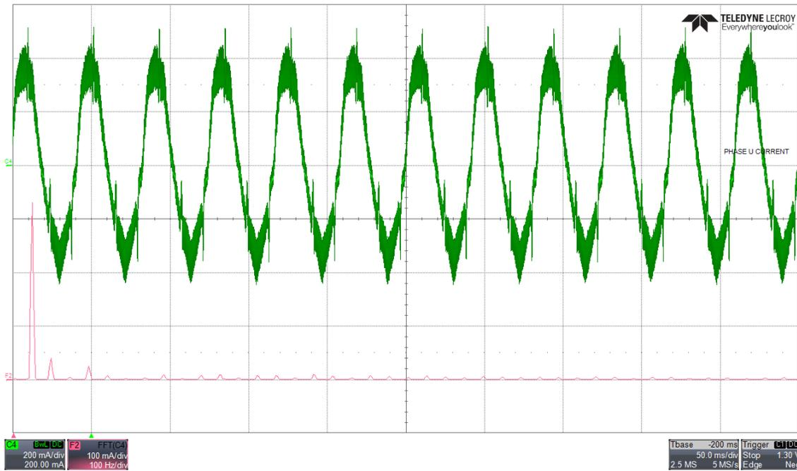
Figure 2-2. Phase current waveform and FFT - Discontinuous PWM modulation
