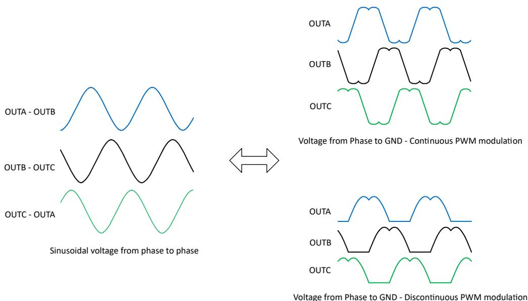
**Figure 2-1. Continuous and Discontinuous PWM Modulation Phase Voltages**
