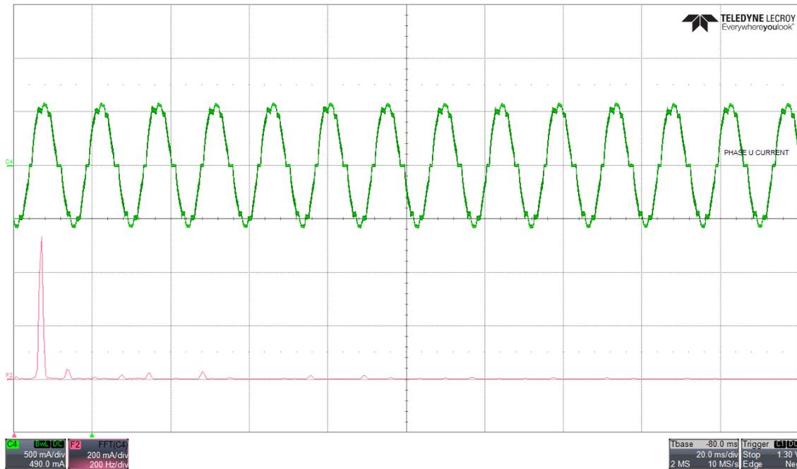
**Figure 2-8. Phase current waveform and FFT - 150° Trapezoidal commutation**
