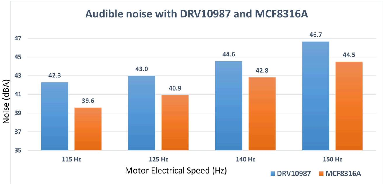
**Figure 2-10. Audible noise comparison between MCF8316A and DRV10987**
