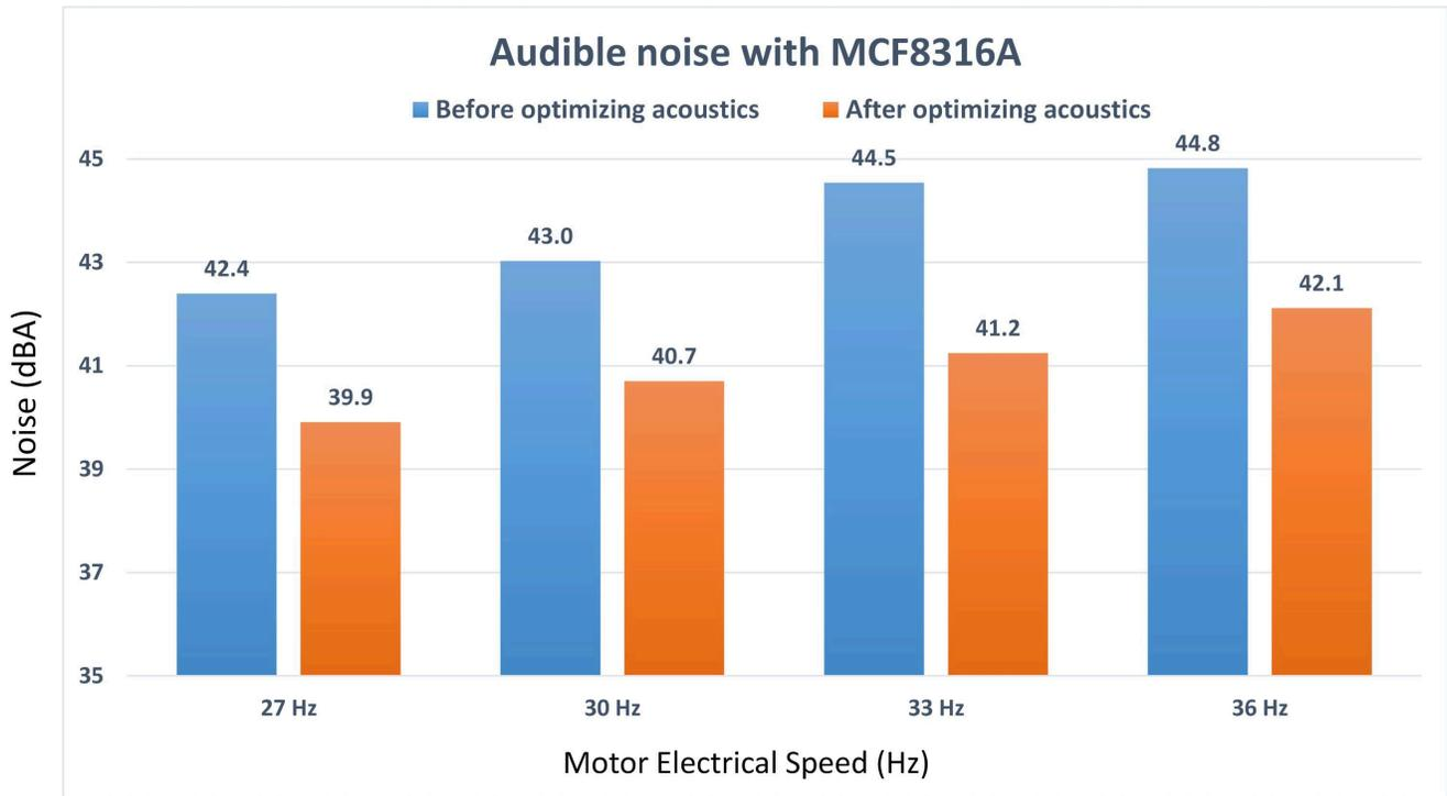
**Figure 2-6. Audible Noise Comparison with MCF8316A**
