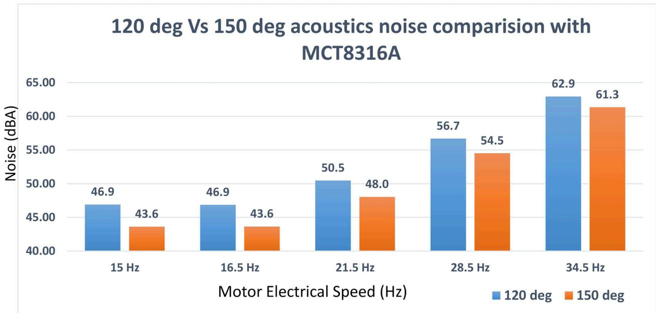
**Figure 2-9. Audible noise comparison between 120° commutation and 150° commutation**
