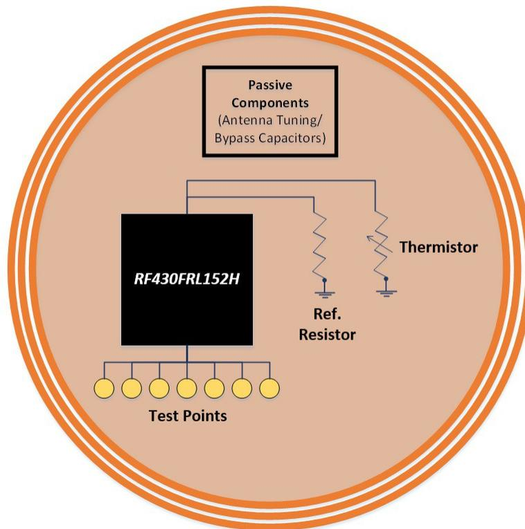
Figure 3. Block Diagram for RF430FRL152 Sensor Tag
