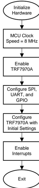
**Figure 6. Hardware Initialization Flowchart**
