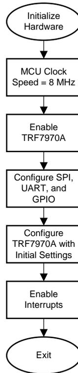
**Figure 6. Hardware Initialization Flowchart**
