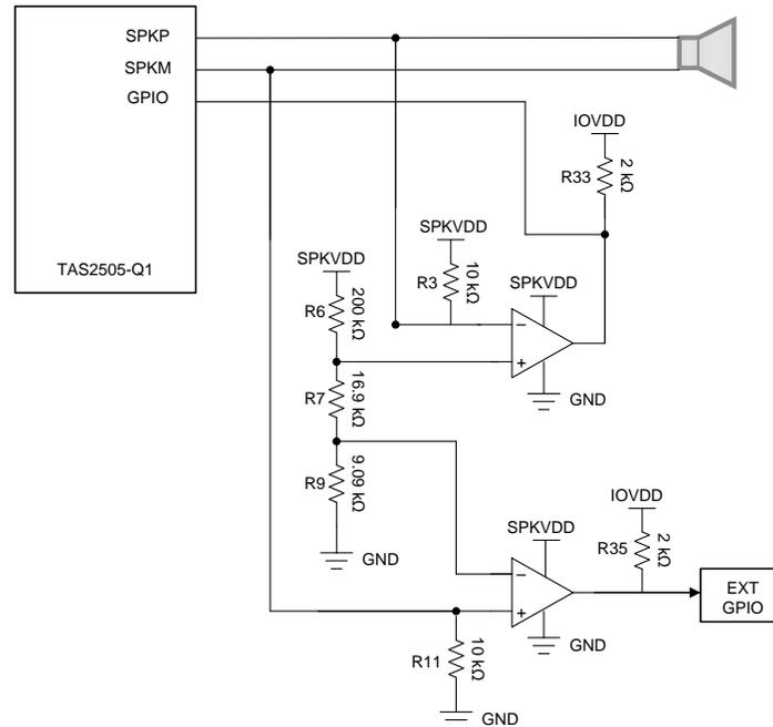
Figure 1. Diagnostic Circuit #1 Schematic
