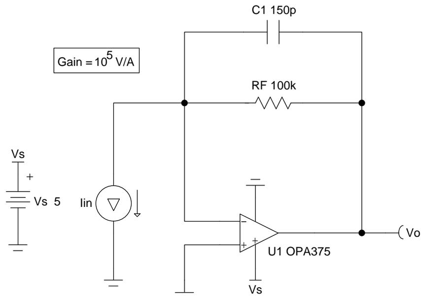
For the circuit in Figure 15, the gain can be calculated using the following equation:
