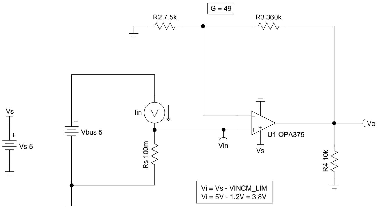
In this example, the gain can be calculated with the following equation:
