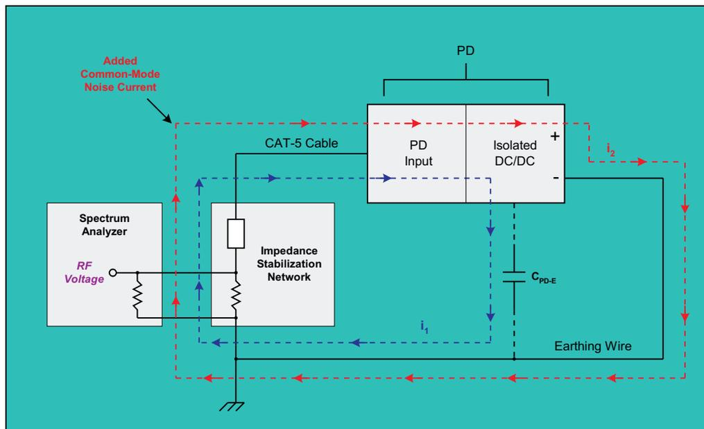
Figure 1-8. Earthed Output Common-Mode Noise Current Path
