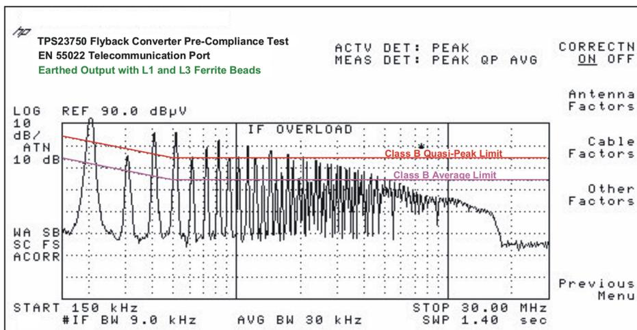
Figure 1-9. Conducted Emissions with Ferrite Beads and Earthed Output
