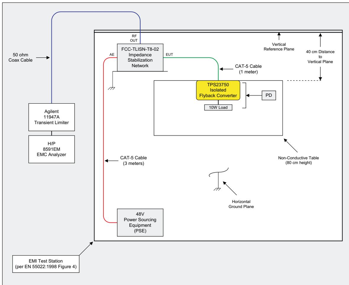
Figure 1-5. Conducted Emissions Pre-Compliance Test Setup Block Diagram
