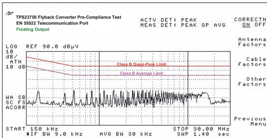
Figure 1-7. TPS23750 Flyback Converter Conducted Emissions Results
