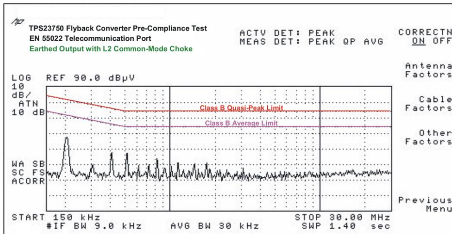
**Figure 1-11. Conducted Emissions with Common-Mode Choke and Earthed Output**
