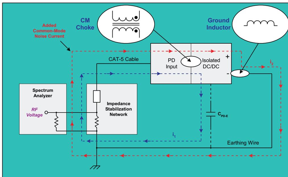
Figure 1-10. Earthed Output Insertion Impedance Options
