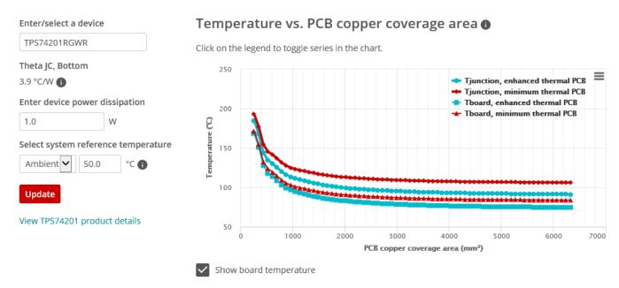
Figure 13. TI PCB Thermal Calculator Example
