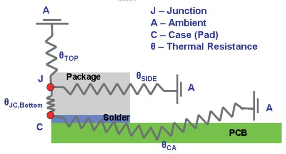
Figure 10. Schematic of Thermal Resistance Network
