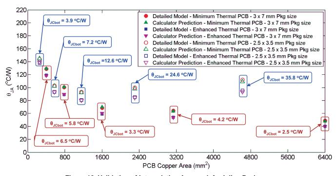
Figure 12. Validation of Interpolation Approach for Inline Packages
