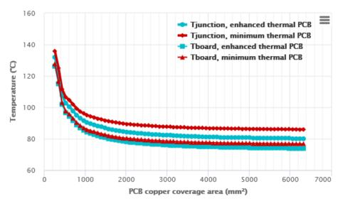
Figure 4. Example Graph Showing Junction Temperature as a Function of Spreading Plane Area for the TAS5701PAP Device at 0.5 W With 65°C Ambient Temperature
