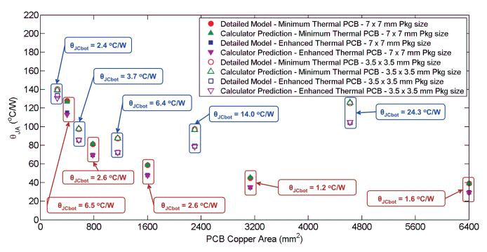
Figure 11. Validation of Interpolation Approach for Quad Packages
