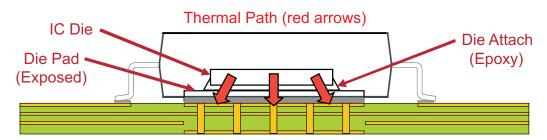
Figure 2. Exposed Pad Package Thermal Path
