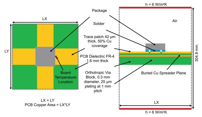
Figure 8. System Model Details for Quad Packages
