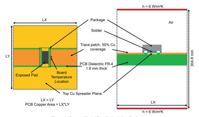
Figure 9. System Model Details for Inline Packages
