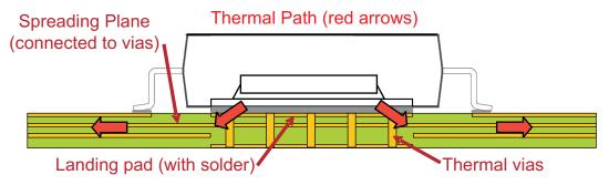
Figure 3. PCB Thermal Path
