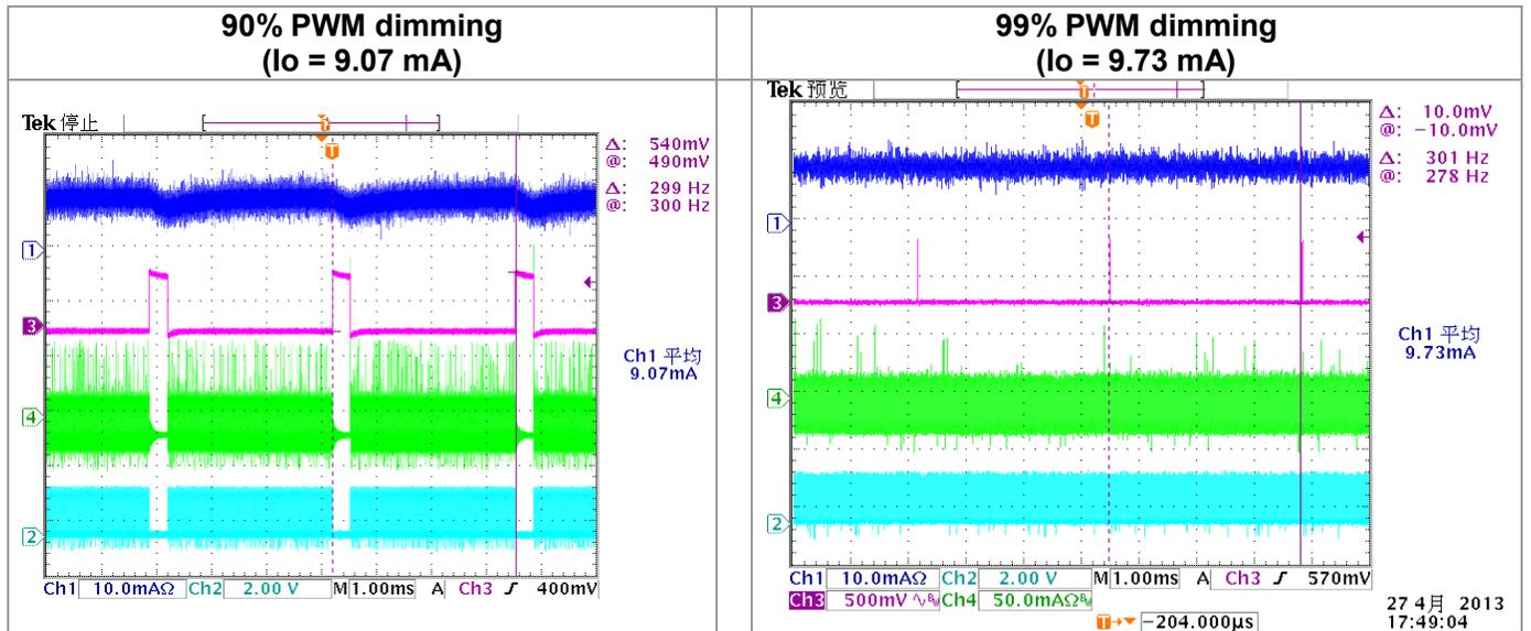
**Figure 17. Measured Waveforms When PWM Dimming is Conducted**
