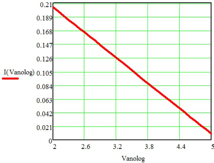
**Figure 9. Calculated Output Current When Analog Dimming**
