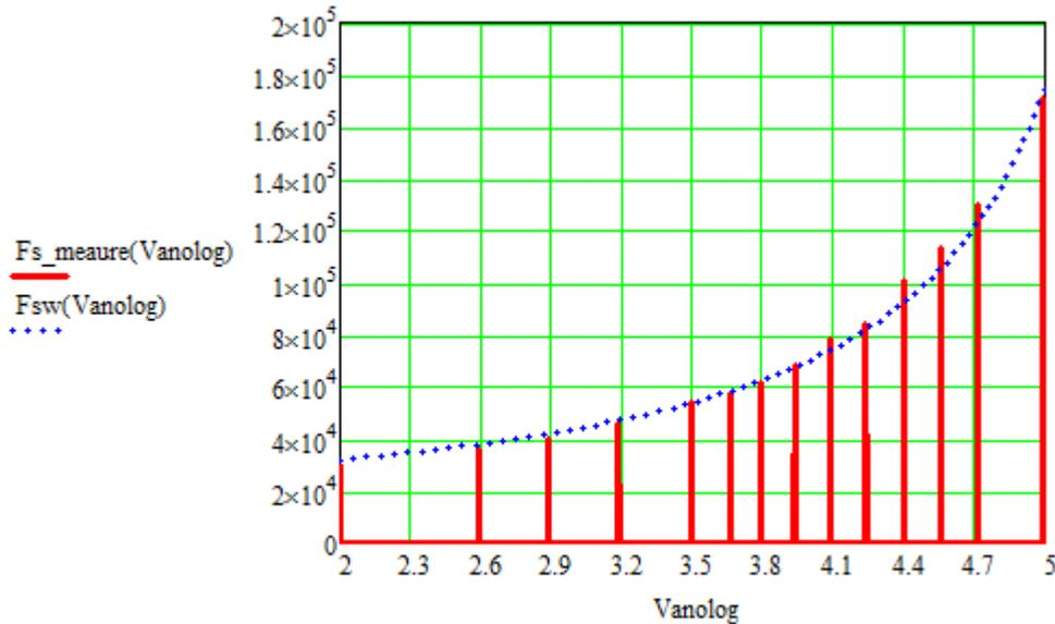
**Figure 15. Operation Frequency Curve—Comparison Between Measurement and Calculation**
