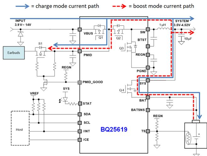
Figure 2. BQ25619 Operation in Charge Mode and Boost Mode
