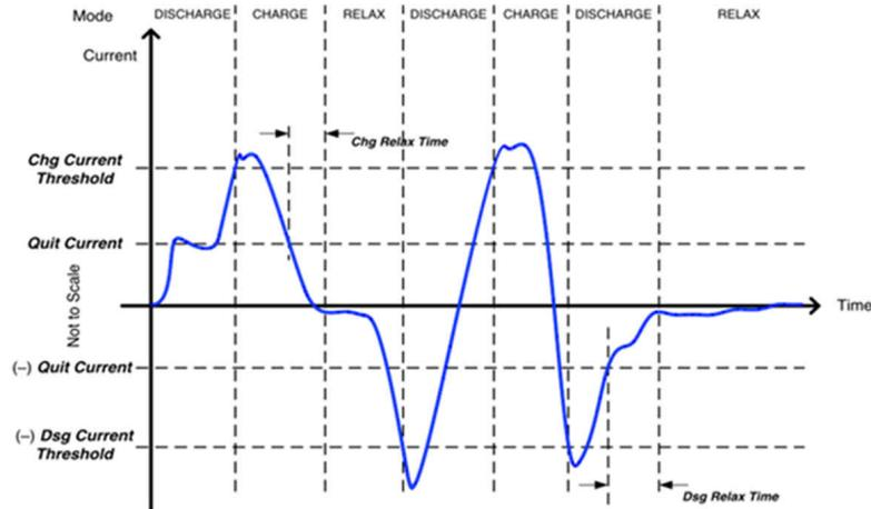
Figure 4-1. Gauge Operating Mode
