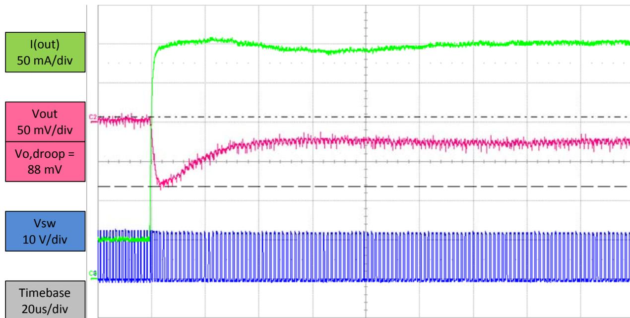
**Figure 4. TPS62125 load transient response from 50-mA to 300-mA load current with a 47- $\mu$ H inductor and a 4.7- $\mu$ F output capacitor**
