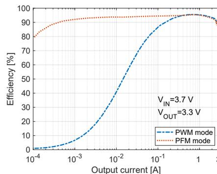
Figure 1-2. TPS63805 Efficiency vs Output Current
