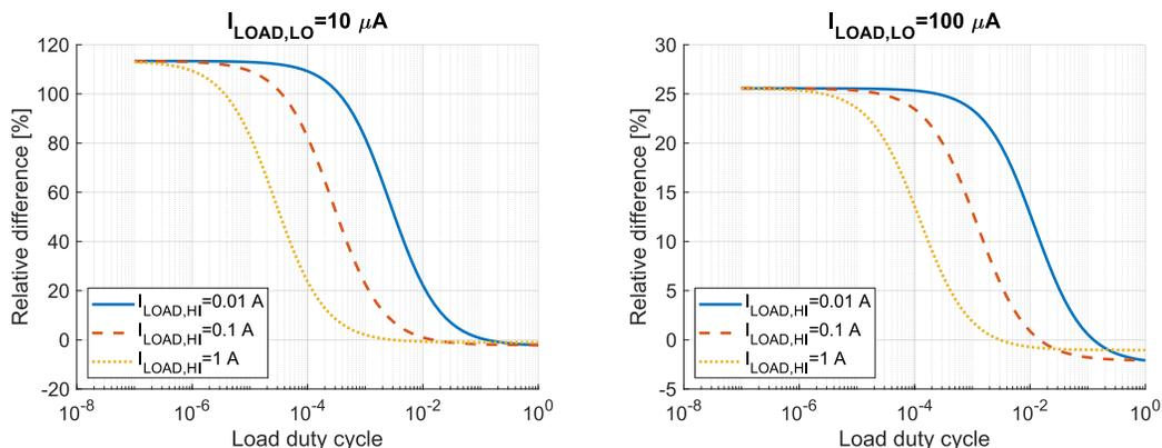
**Figure 2-1. Relative Difference in Battery Consumption vs Load Duty Cycle**
