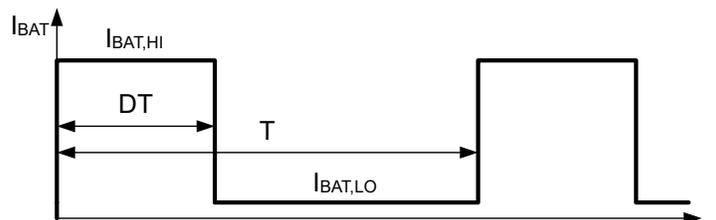
Figure 1-1. Battery Current Profile with a Pulsed Load
