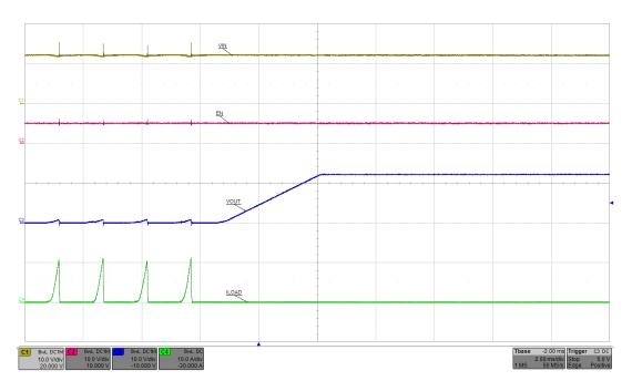
Figure 15. Recovery From Output Short Circuit
