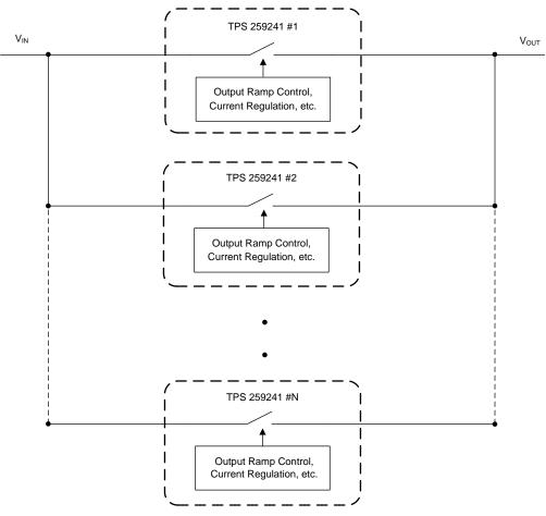
Figure 2. Number of "N" eFuse Devices Connected in Parallel Configuration
