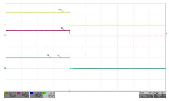
Figure 8. Current Profile of Two Devices During Shut-Off
