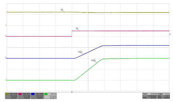
Figure 9. Load Turn-On Behavior of 20-A eFuse With Enable-On
