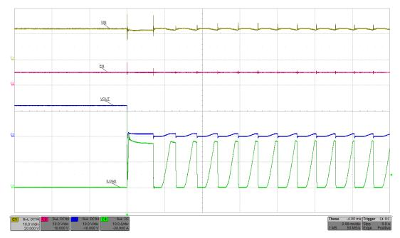
Figure 14. Output Short-Circuit Response of 20-A eFuse
