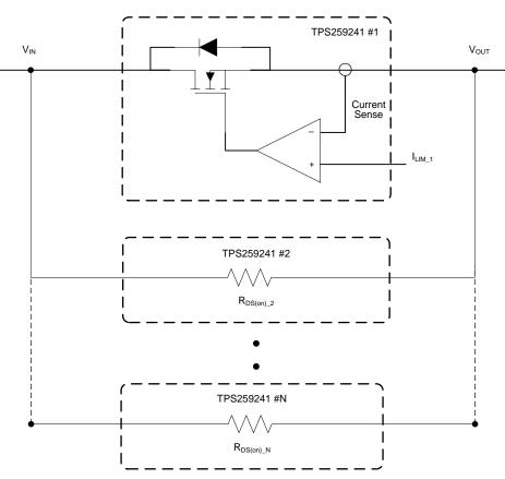
Figure 4. Equivalent Circuit of Parallel-Connected eFuses When One Device Reaches Current Limit
