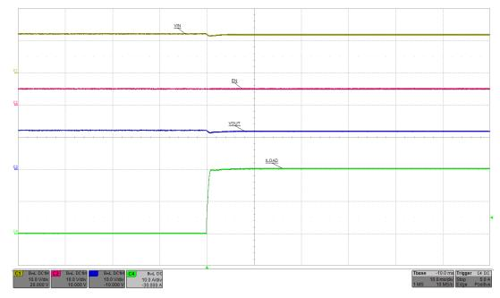
Figure 11. 20-A Load Step-Up Response of Four-Phase eFuse Parallel Configuration
