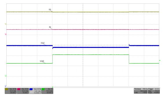
Figure 13. Transient Overload Response of 20-A eFuse
