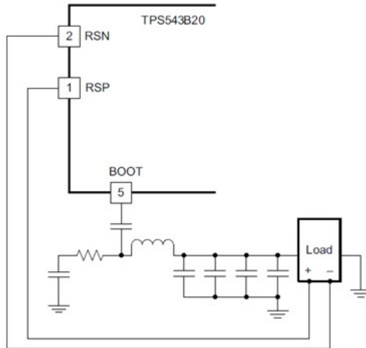
Figure 7. Remote Sense With Feedback Resistors
